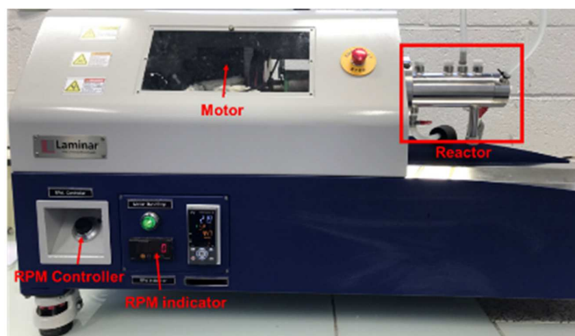
Figure IV-4 : Photo of the whole Couette Taylor apparatus implemented in the laboratory.
