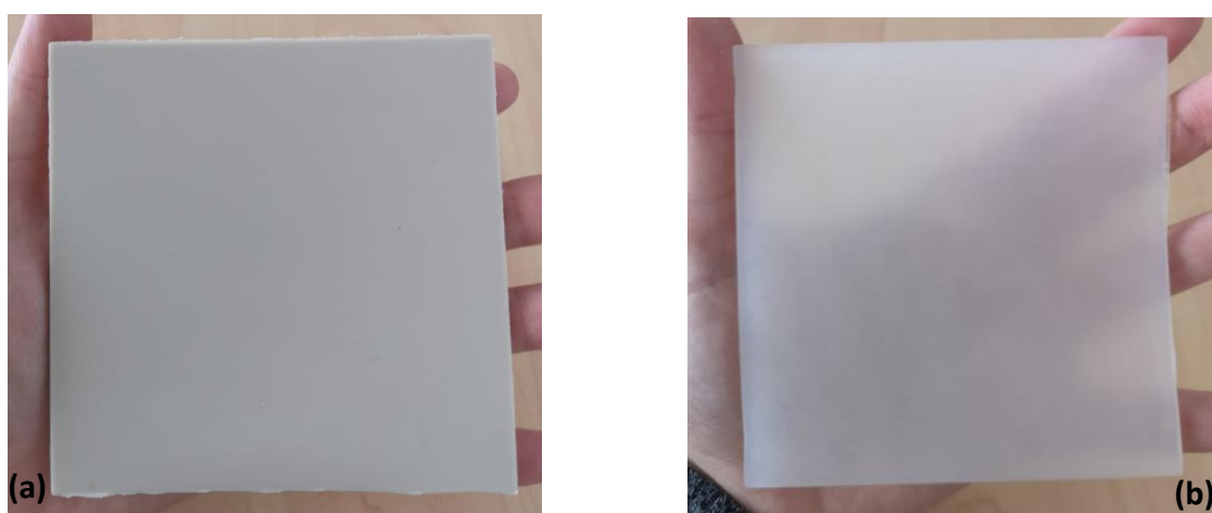
Figure 31: 100×100 mm 2 Plaques of a) Filled PVC; b) Unfilled PVC
