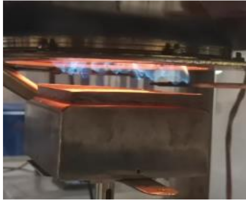
Figure 72: Premixed flame during PMMA burning at 13 vol. % of oxygen
