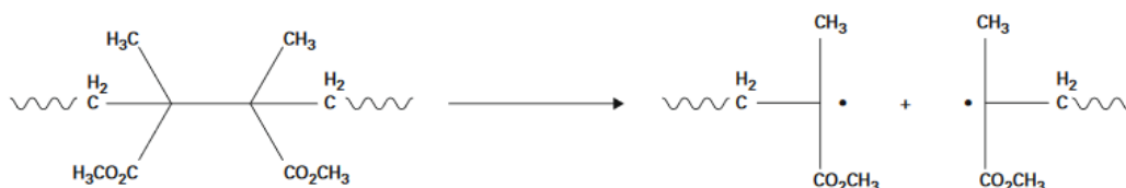
Figure 2: Thermal decomposition of a free radical polymerized of PMMA [12]
