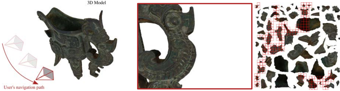
Figure 1.16 – An example of user’s navigation around the 3D model (left), what he observes at a given instant (center), and the corresponding visible blocks \mathcal{V} (in red) in the atlas (right). For better visibility of the blocks, the black background area is turned into white in the atlas.
