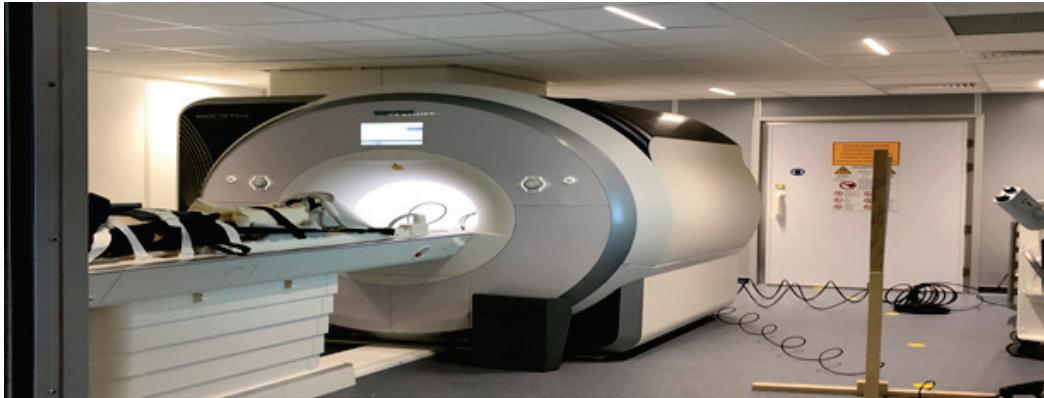
Figure 5.1.: Installation setup of the patient or volunteer. She/he would lay down supine, her/his foot attached to a pedale ergometer Trispect module. An additional screen not shown here was behind the patient, and that is where instructions were displayed thanks to the e-Primes software.
