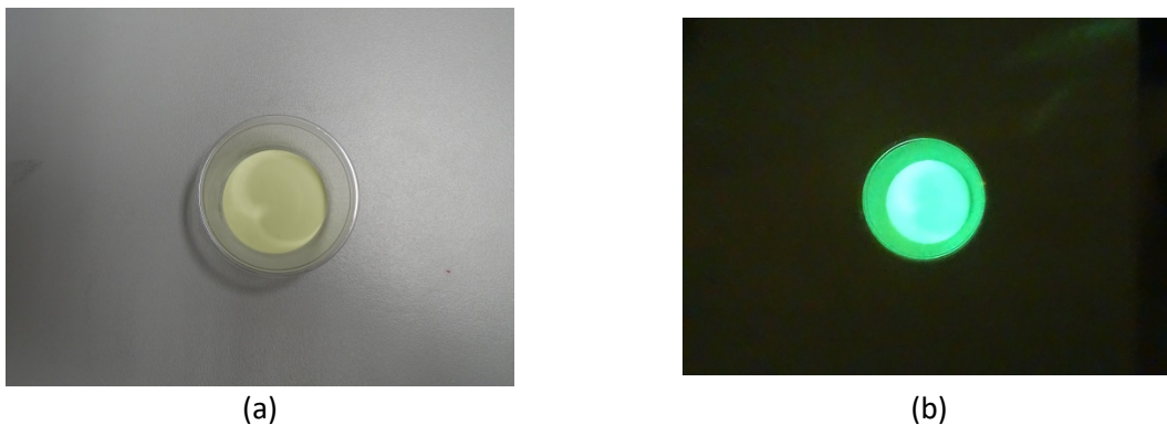
Figure 2.2: Pigment Lumilux ® Green SN-F50; a) in ambient light, b) in dark room.
