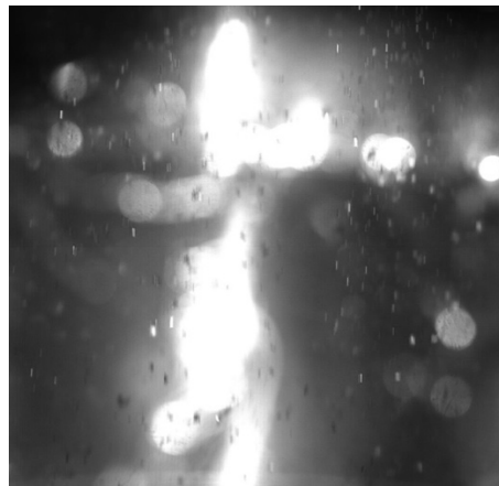
Figure 2.4: Flow concentration of SiC-Pigment particles in activation part.
