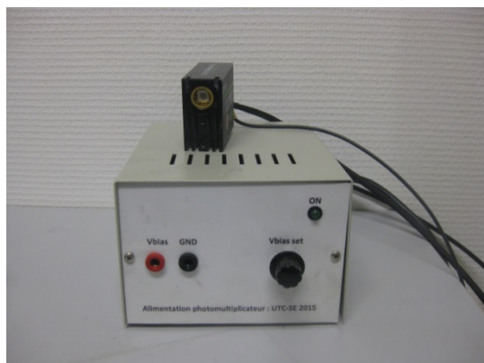
Figure 2.12: Supply system and PMT.
