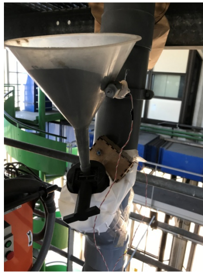
Figure 3.2 : Schematic of the solid feeding system.
