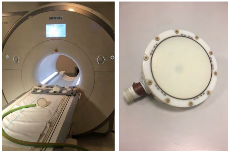
Figure 2.11 Left side: Custom-made MRE pneumatic MRE passive driver on the table of the 1.5 T MRI scanner (MAGNETOM Aera, Siemens). The mechanic exciter is connected to a subwoofer speaker with a plastic hose. Right side: detailed view of the 3D-printed pneumatic MRE passive driver.
