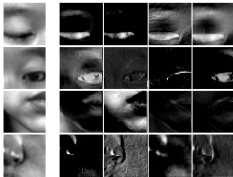
Figure 5.5: Filters responses at convolutional layer number 2. The first column on the left represents the original patch.
