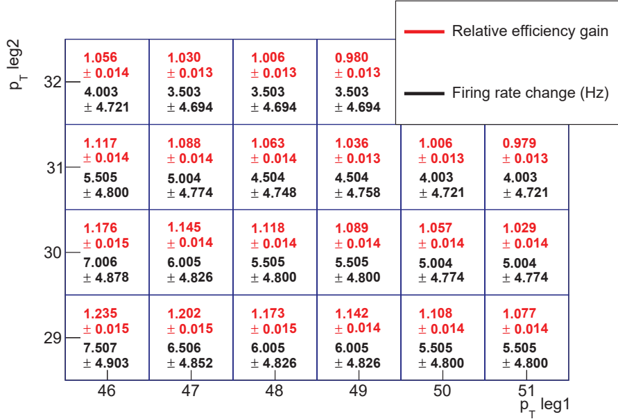
Figure 4.1: Values of the relative efficiency gain and the firing rate increase for different values of p_T thresholds. The displayed uncertainties are only statistical. The complete studied range was 35 to 60 GeV for the leading HLT \tau_h object and 20 to 40 GeV for the sub-leading, but only the region that was found to be most interesting in terms of efficiency gain and rate increase is displayed here.
