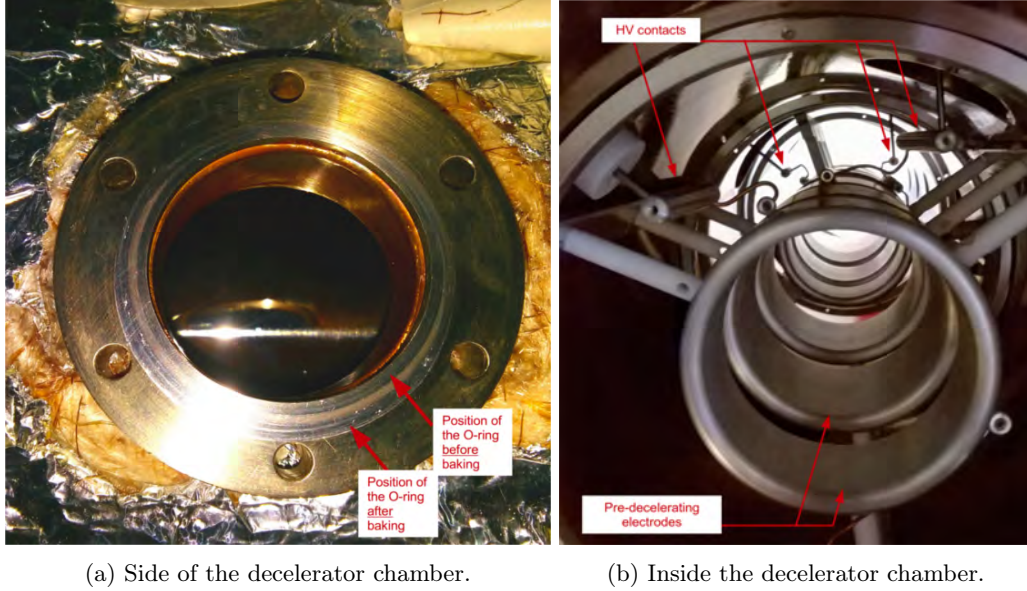
Figure 5.25 ( left ) - Picture of a flat port on the side of the in-line decelerator chamber after baking at 200^\circ . The mark of the Helicoflex O-ring before and after the baking are visible. ( right ) - Picture of the inside of the in-line decelerator chamber with the high voltage in-vacuum connections. The in-vacuum connections appear on the top of the picture for the pre-decelerating electrodes.
