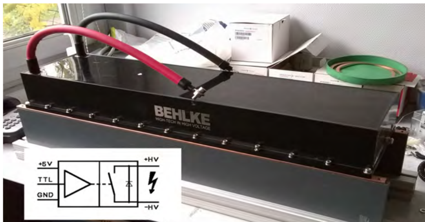
Figure 5.9 Picture of the BEHLKE HTS 1501-20-LC2 single pole, single throw (very) high voltage switch. The switch is presented mounted on insulated plastic supports.
