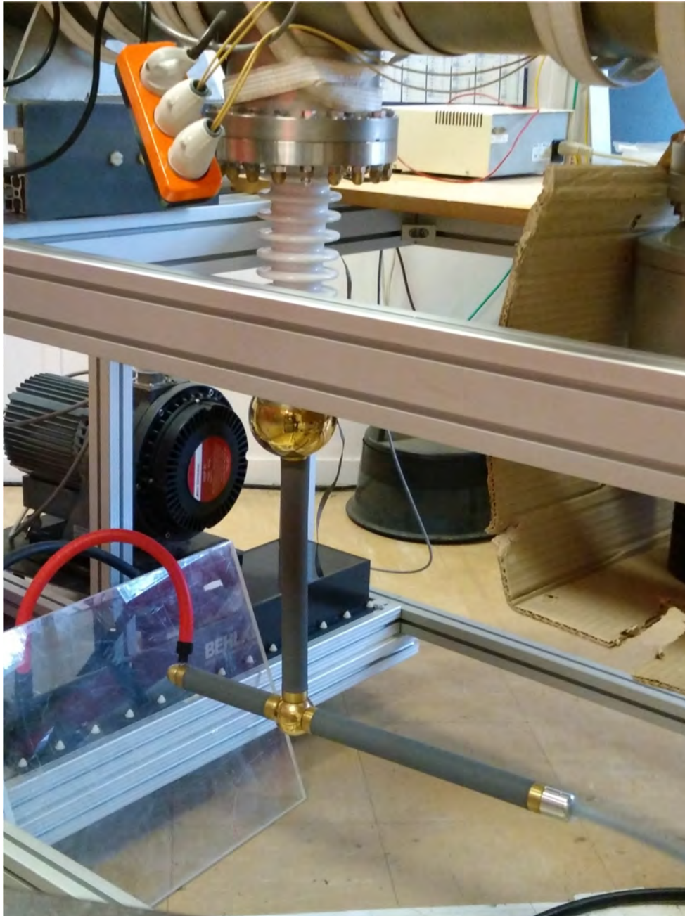
Figure 5.13 Picture of the high voltage assembly in the SPST configuration. The grey bars are the high voltage ceramic resistors. The cable on the right provides the 100\text{ kV} tension. The circuit is connected on the upper part through the white ceramic feedthrough to the drift tube. In the background on the left, behind a Plexiglas plate, the SPST switch is connected to the system on one branch and to the earthed chassis on the other one. The feedthrough connection is made inside a hollow brass ball to avoid corona.
