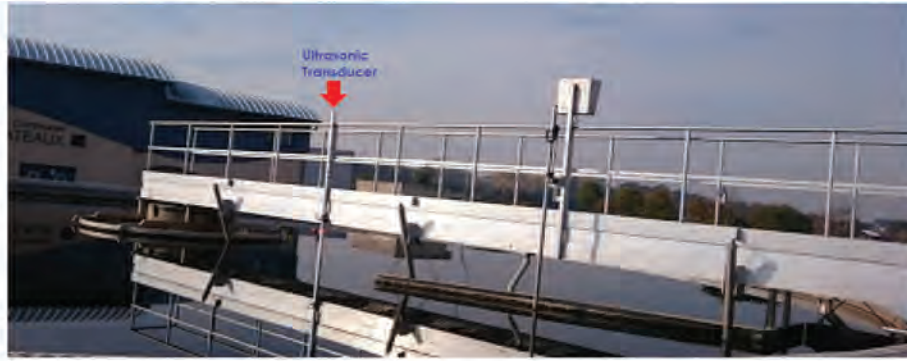
FIGURE 4.6: Overview of the support and Peacock UVP system placed in the clarifier
