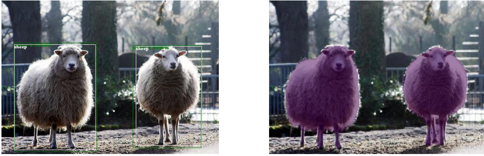
Figure 1.3 – An example of an image annotated for object detection (left) and semantic segmentation (right). In this simple case solving semantic segmentation automatically leads to solving object detection. On the other hand, providing bounding boxes gives a very strong clue for semantic segmentation.
