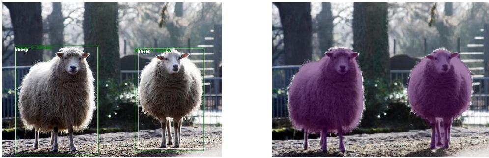
Figure 3.1 – The outputs of our pipeline. On the left, the bounding boxes were generated as a solution for object detection. The right image shows generated class maps for semantic segmentation.
