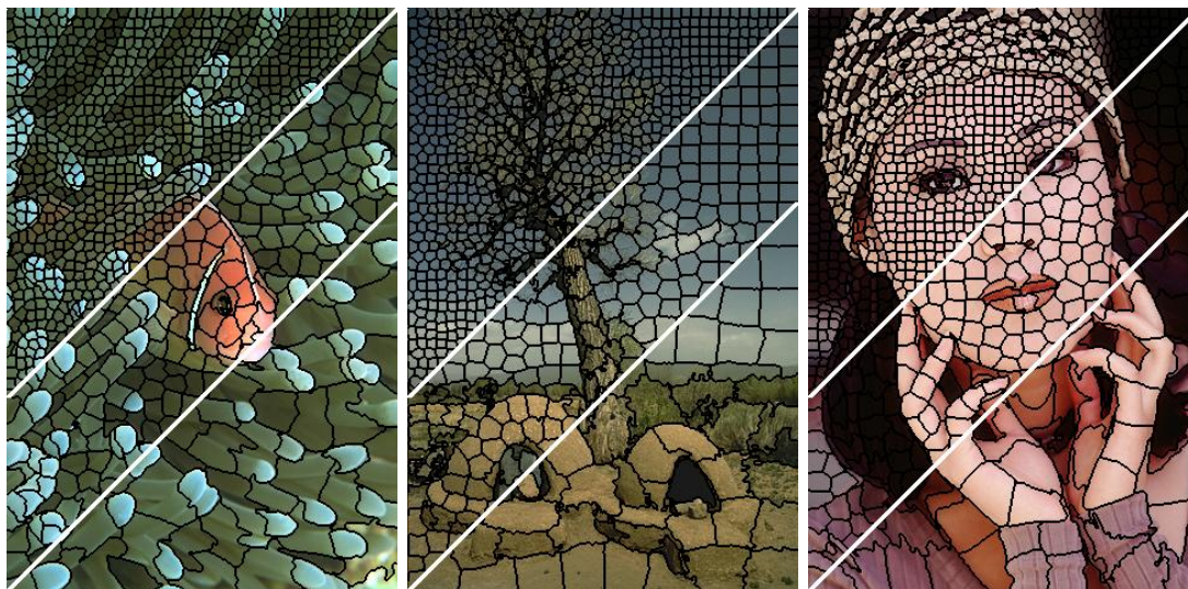
Figure 2.4 – Superpixels are groups of neighboring pixels organized together at several scales based on their color and gradient similarity. Image source [3].
