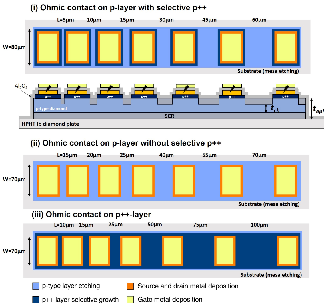
FIGURE 5.2: Top view and side view of the mask used to fabricate the structures measured to analyse the diamond resistivity and contact resistance.
