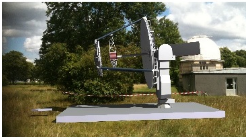
Figure 12: Rendering of the GATE project, prototype for the small-size-telescopes in the CTA array. The main mirror has a diameter of four meters
