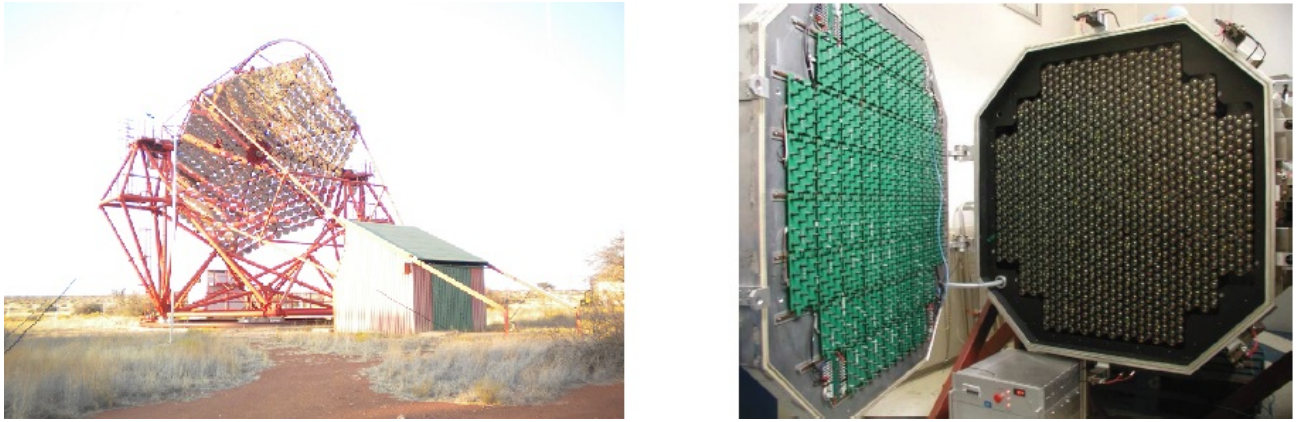
Figure 4.1: Left : view of one of the H.E.S.S. telescopes, showing the structure, the segmented mirror (in the left part can be seen a missing mirror, replaced by the CCD camera used for the pointing corrections), and the building covering the camera during day-time. Right : view of one of the H.E.S.S. cameras, showing the cover (on the left), equipped with a LED panel, used for the calibration of the PMs. Taken from Guy (2003).
