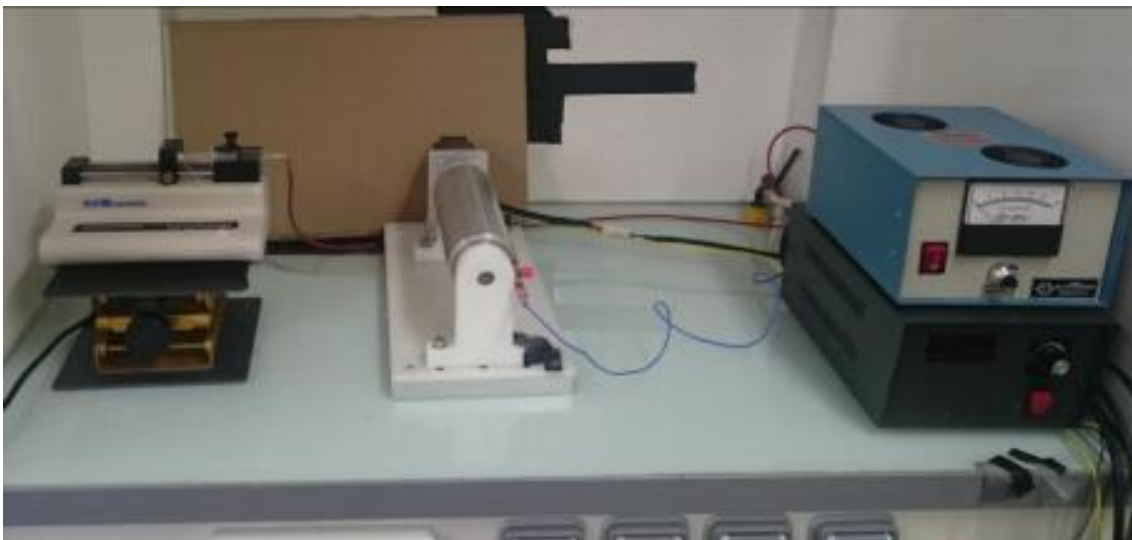
Figure 5. Electrospinning device of Laboratoire Roberval.
