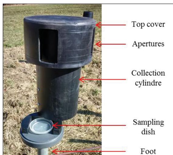
Figure 2.1. Picture of the passive SIGMA-2 dust collector
