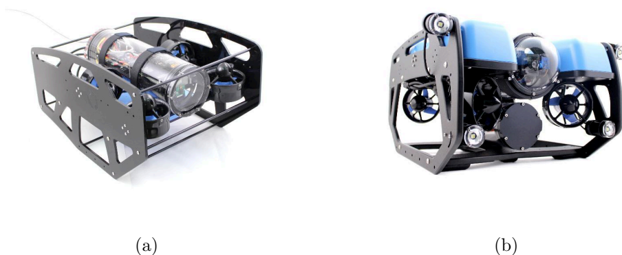
Figure 2.3: The experimental robots used in this thesis: (a) the BlueROV1 and (b) the BlueROV2, both from Blue Robotics.
