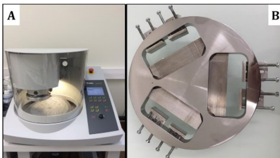
Figure 66. A) Polishing set Tegramin-30 ( Struers ); B) sample holder, adapted for large samples surfaces preparation.
