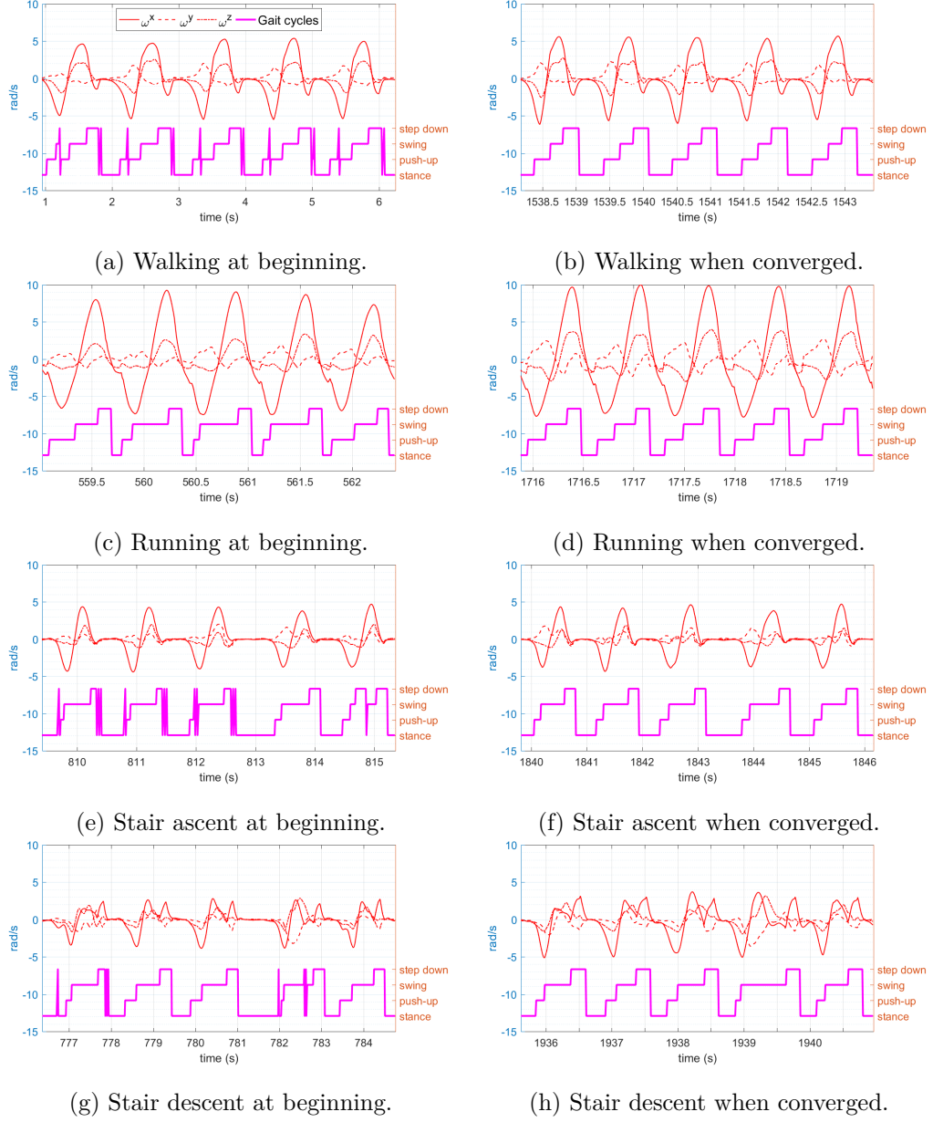
Figure 4.12: The detected gait cycles at the beginning of each activity (left column) compared to the ones when the estimation of the model's parameter has converged (right column).
