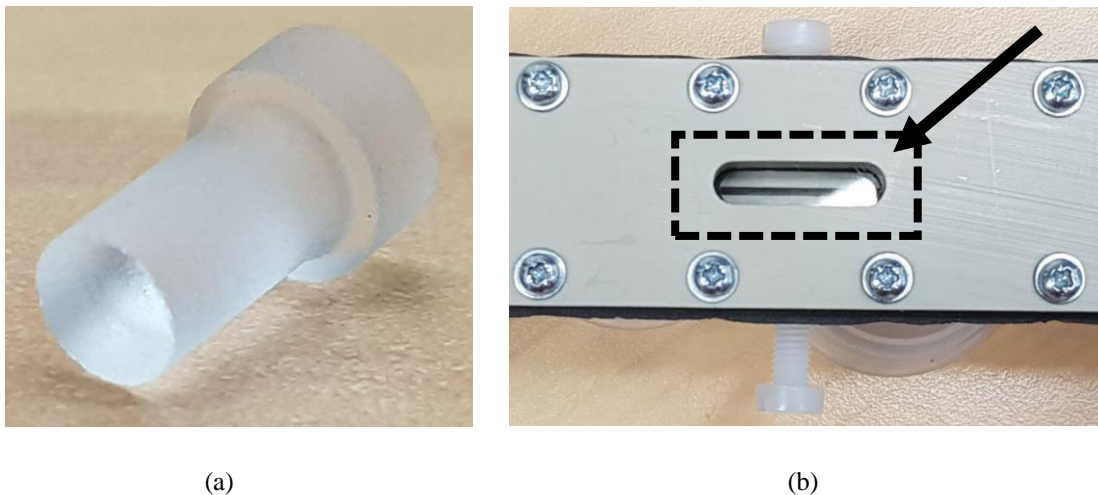
Figure 4.38. (a) Suprasil® window; (b) Borosilicate optical access for ICCD acquisition. The smaller dimension of the rectangular gap that can be seen through the window corresponds to the height of the channel.
