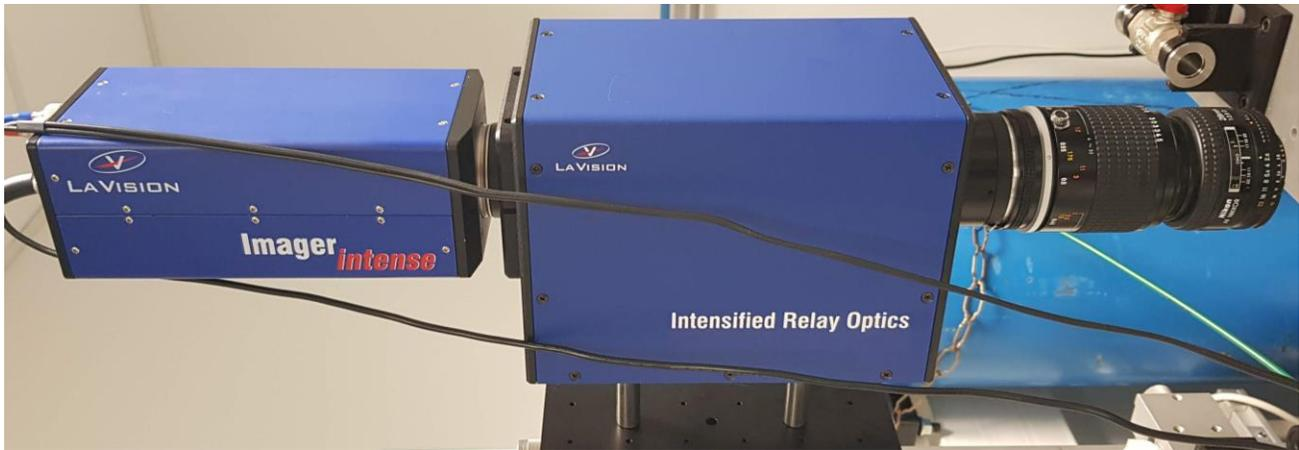
Figure 4.14. Acquisition system ICCD.
