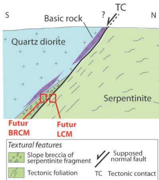
Figure 4. An example of hypothetical tectonic context consistent with the formation of serpentinite breccia that serves as receptacle for mineralization. In that case, fault motion need to be normal. (BRCM: Brecciated-related contact mineralization; LCM: Laminated contact mineralization)
