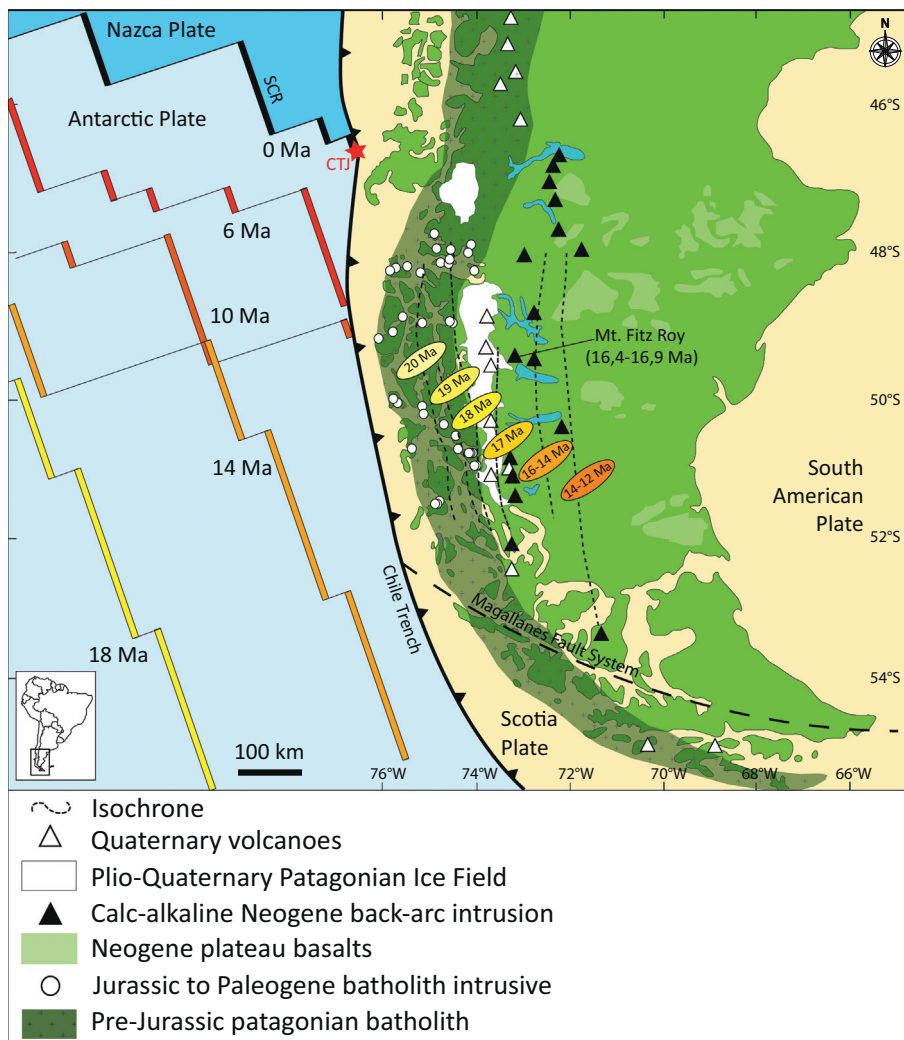
Fig. 10. Simplified geological map of Southern Patagonia showing the location and age of the Miocene magmatic arc (after Espinoza et al., 2010; Ramírez de Arellano et al., 2012). The present-day location of the South Chile Ridge (SCR) is indicated in black, and the red star indicates the present-day position of the Chile Triple Junction (CTJ), west of the Taitao Peninsula. Red to yellow lines represent past locations of the Chile Ridge segments with respect to South America at 6 Ma, 10 Ma, 14 Ma and 18 Ma, respectively. Dark green area along the western border of the continent indicates the position of the Southern Patagonian Batholith (Pankhurst et al., 1999; Hervé et al., 2007). Light green areas in the central and eastern part of the South American continent correspond to the Neogene Patagonian plateau basalts, with ages ranging from 12 to 7 Ma in the western part of the back-arc and from 5 to 2 Ma farther to the northeast (Gorring et al., 1997). Dashed lines on the continent show the Miocene eastward migration of the magmatic arc (after Espinoza et al., 2010 and Ramírez de Arellano et al., 2012). Small white circles correspond to Jurassic to Paleogene batholith intrusives. Black triangles are calc-alkaline Miocene plutons (see references in Espinoza et al., 2010 and Ramírez de Arellano et al., 2012). White triangles are the Quaternary volcanoes (Stern and Kilian, 1996). (For interpretation of the references to color in this figure legend, the reader is referred to the web version of this article.)
