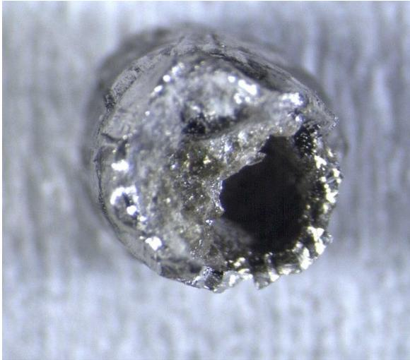
Figure D2: Recovered Pt capsules for PC133-1 at the opening big holes indicating massive degassing. Capsule diameter is 3 mm.
