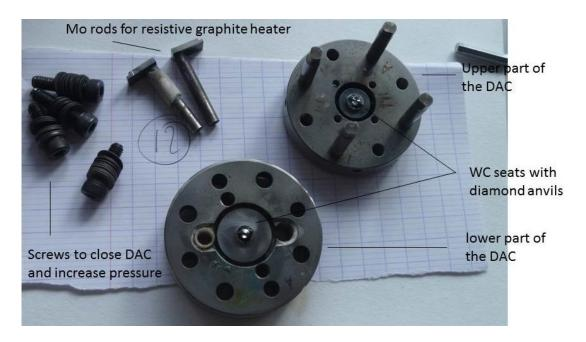
*Figure C6: Example of DAC from P02.2 team, DESY, Hamburg. Design with two symmetric parts, each having a WC seat with a diamond anvil.* P *is increased by closing the cell and screwing the two parts toward each other.*
