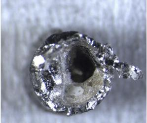
Figure D2: Recovered Pt capsules for PC133-1 at the opening big holes indicating massive degassing. Capsule diameter is 3 mm.
