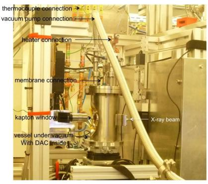
Figure C10: Experimental set-up on P02.2 (beamline at DESY, Petra III, Hambourg, Germany) for graphite heater. DAC is disposed inside a vacuum vessel to prevent oxidation of Mo rods, WC seats and diamonds. Maximal T is 1700 K.
