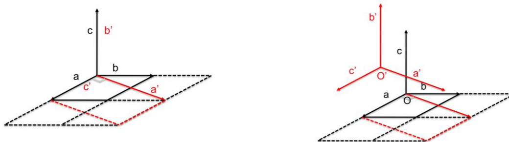
Figure E4: Operations to pass from hexagonal \beta -quartz structure (in black) to orthorhombic structure (in red).
