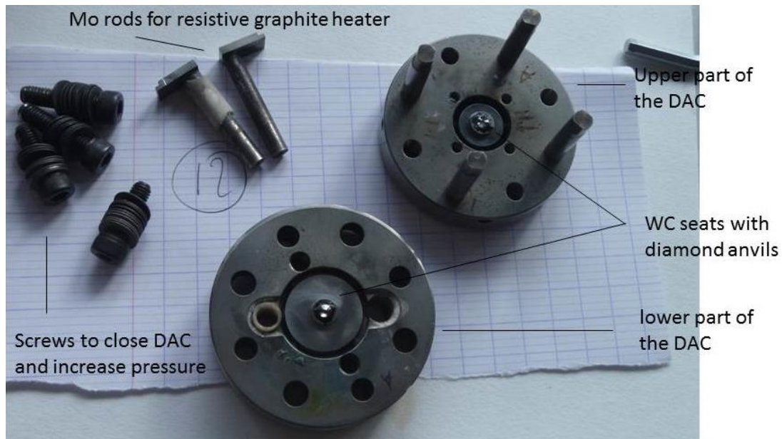
Figure C6: Example of DAC from P02.2 team, DESY, Hamburg. Design with two symmetric parts, each having a WC seat with a diamond anvil. P is increased by closing the cell and screwing the two parts toward each other.
