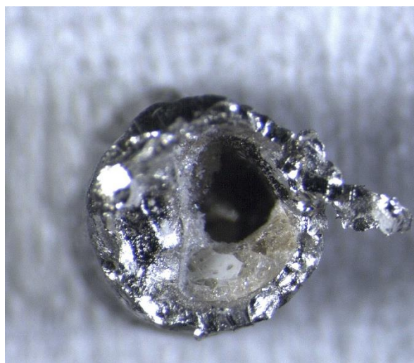
Figure D3: Recovered Pt capsules for PC135-1 at the opening big holes indicating massive degassing. Capsule diameter is 3 mm.
