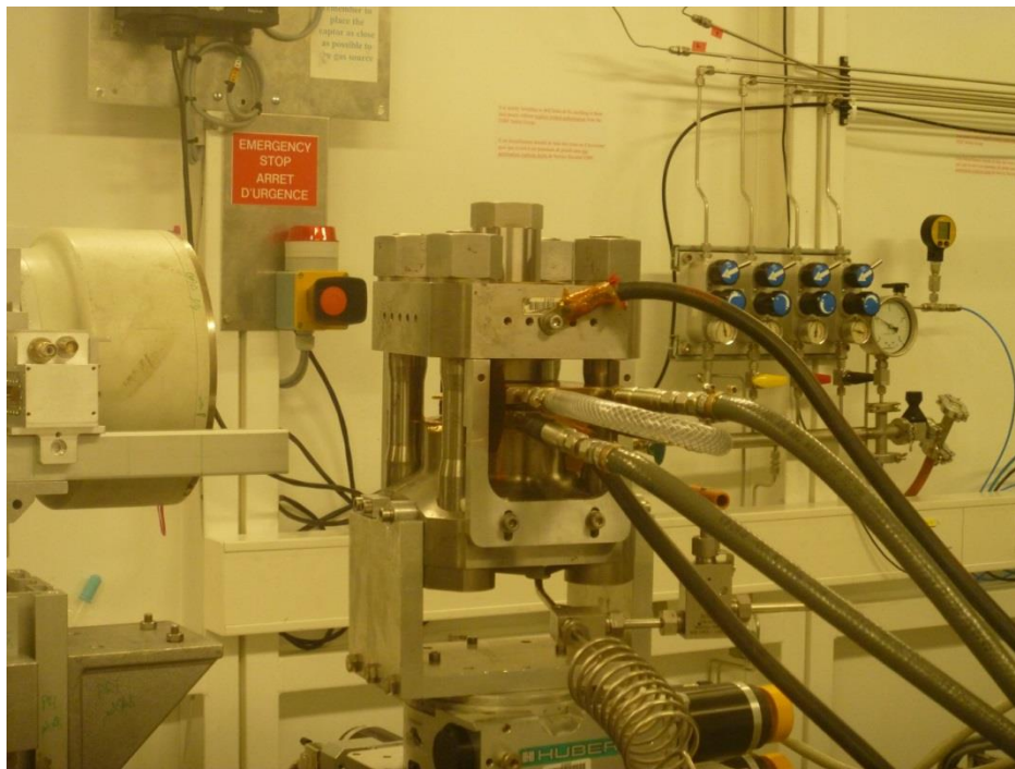
Figure C11: Experimental set-up with PEP on beamline BM23, ESRF (European Synchrotron Radiation Facilities). Black cables are furnace connections and grey transparent tube is water cooling system. On the left side: MAR image plate (area detector to record X-ray diffraction pattern).
