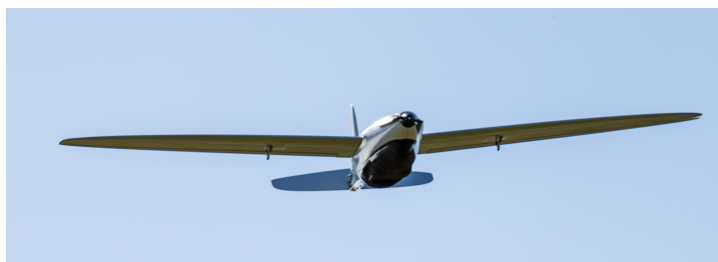
Photograph of Cumulus One in deep-stall flight (Courtesy Sky-Watch A/S).
