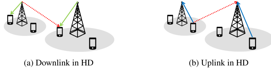
Fig. 1.2 Interference created in HD-based networks, where the red-dotted lines represent an interfering link. For the downlink in (a), the interference is generated by other DLs (transmitting BSs). For the uplink in (b), the interference is generated by other ULs (transmitting UEs).
