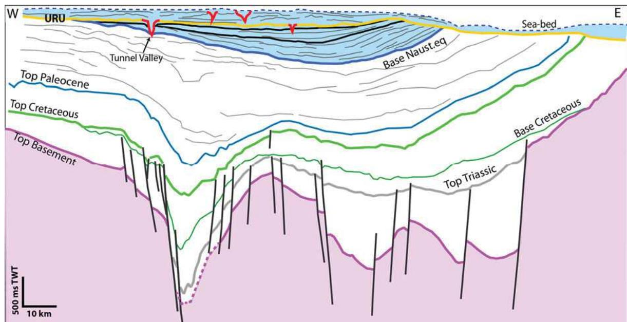
**Figure V-2.** Geological cross-section across the central Viking Graben (compiled from Ottesen et al., 2014 and Evans, 2003; see Figure V-1 for location). Note that mid to upper Pleistocene tunnel valleys (in red) have incised down to the early Quaternary sediments beneath the Upper Regional Unconformity (yellow line; Stewart et al., 2013; Ottesen et al., 2014, 2018). URU: Upper Regional Unconformity.
