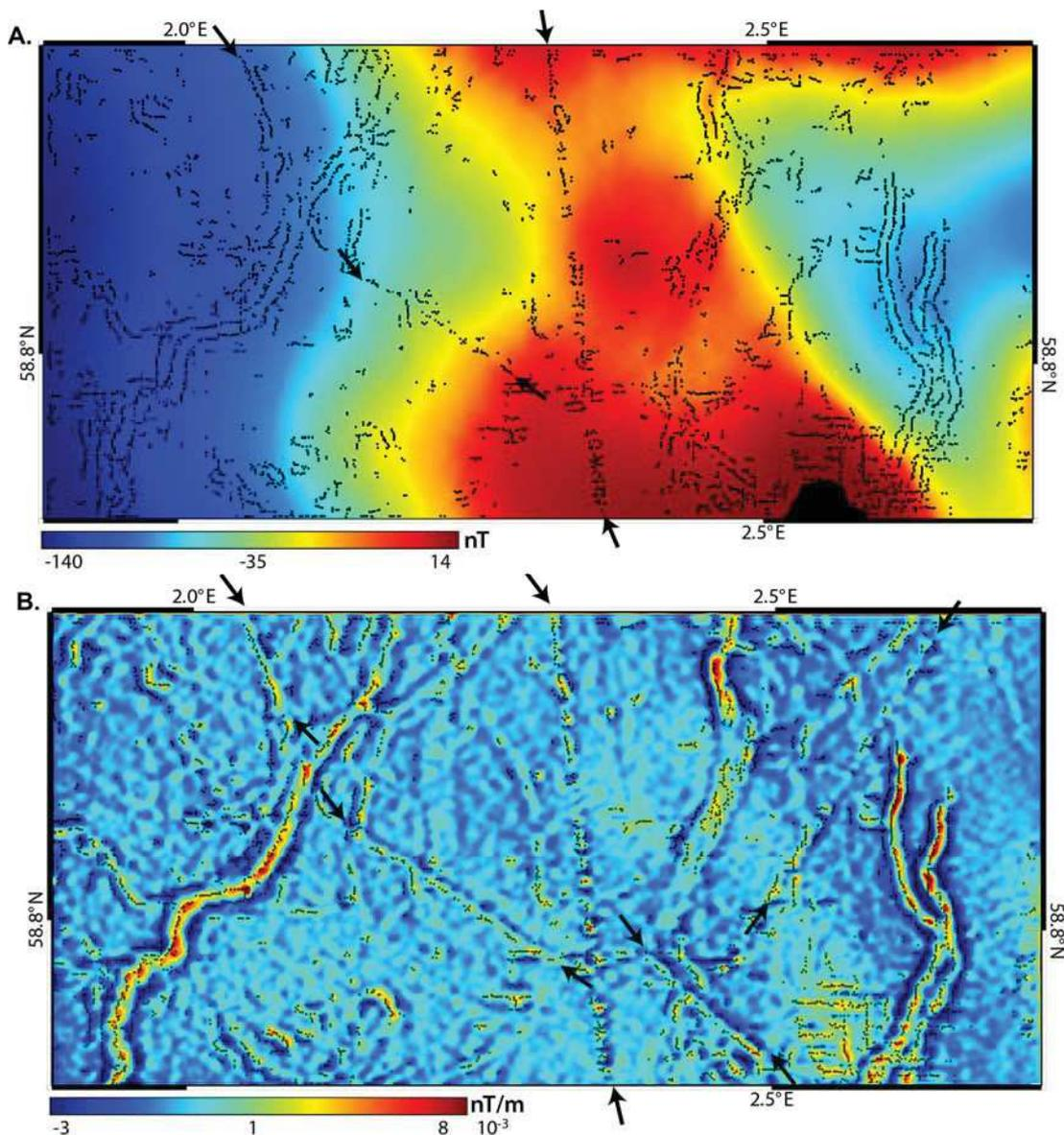
**Figure V-5.** Plotted maxima of the horizontal gradient on (a) the TMI, and on (b) the order 1.7 vertical derivative map (see Fig. V-3a for location). Black arrows show straight lineations representative of non-geological structures (ex. Pipeline).
