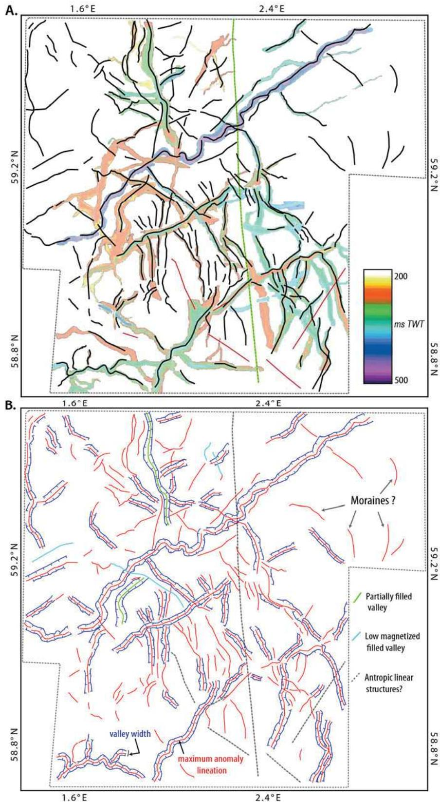
**Figure V-11.** Correlation magnetic and seismic tunnel valley analysis. (a) Map showing the correlation of the seismic tunnel valley and the magnetic anomaly lineations extent; black lines correspond to the maxima of vertical derivative magnetic anomalies; (b) Generalized tunnel valley widths.
