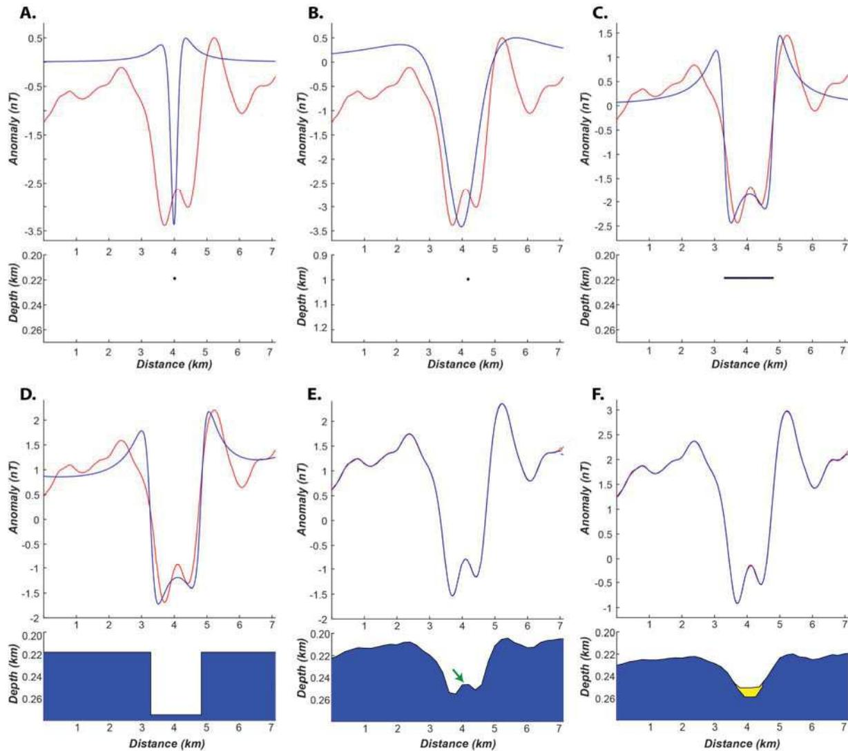
**Figure V-9:** Results of magnetic 2D forward modeling applied to an unfilled valley using (data: red curve, model: blue curve): (a) shallow cylinder; (b) deep cylinder; (c) horizontal finite-width plate; (d) rectangular shape; (e) iterative inversion; green arrow shows positive relief at the incision bottom, not corresponding to a bathymetric feature (Fig. V-7c); (f) iterative inversion of data minus the magnetic effect of the polygon under the bathymetric incision (yellow polygon).
