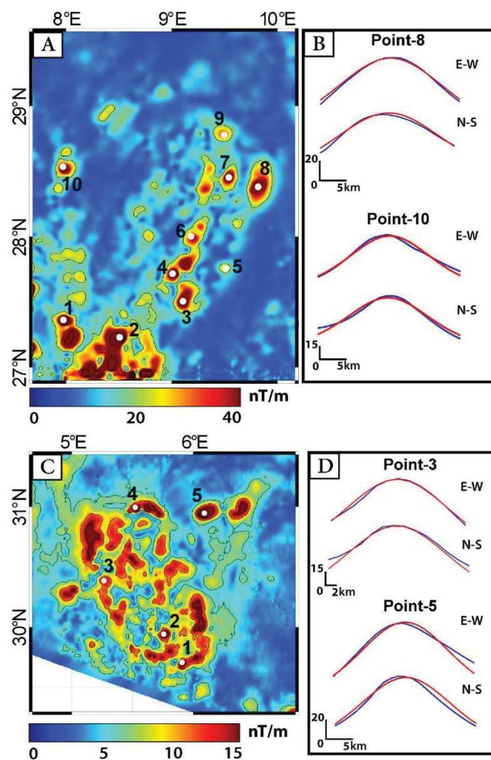
**Figure III-6:** Distribution of the analytic signal maxima in (A) the northern part of UC1 and (C) in the northern part of UC3; (B & D) selected examples of profiles showing the result of the analytic signal inversions (Analytic signal in red, modeled signature in blue). See Table 2 for computed depths.
