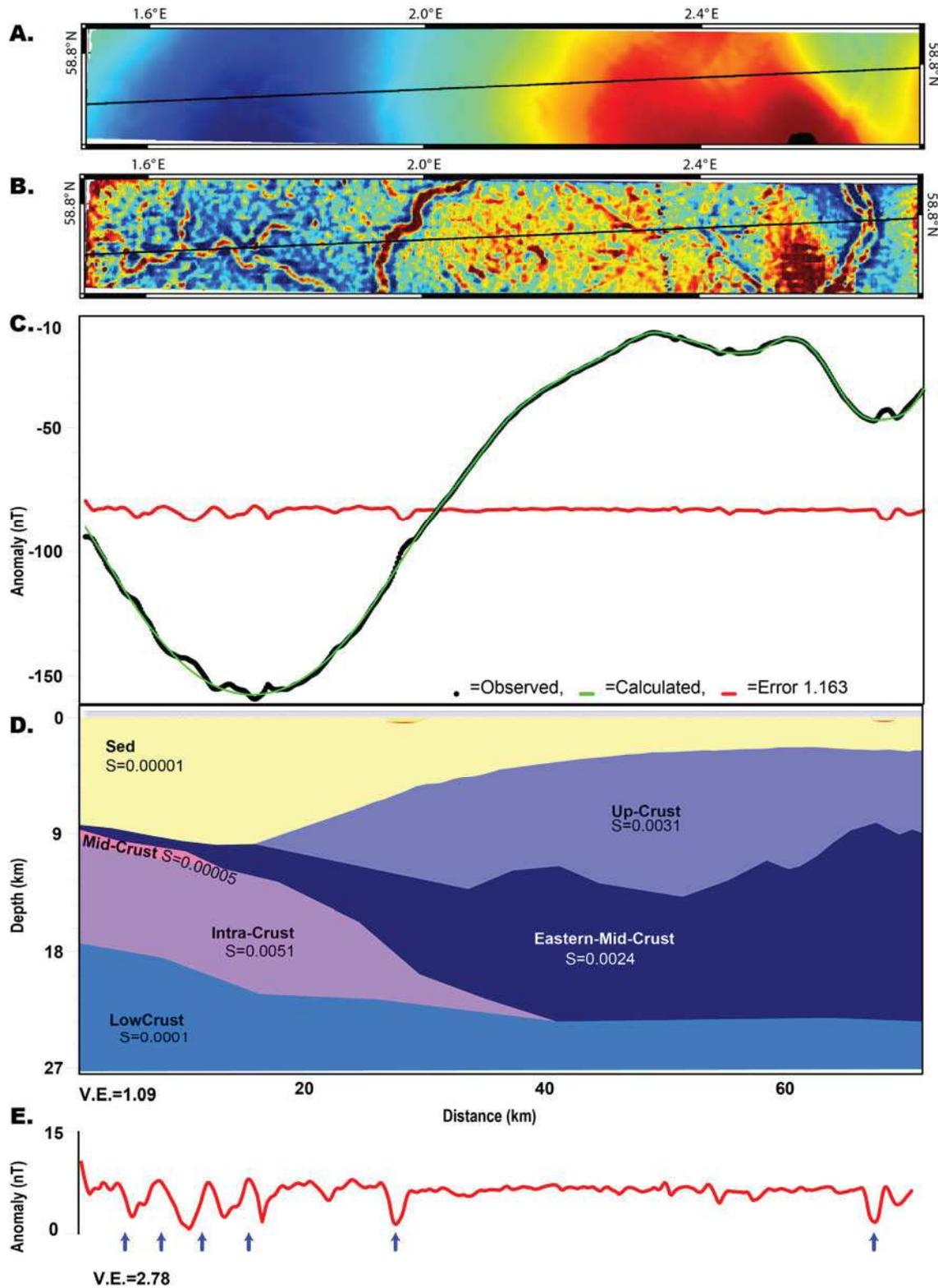
**Figure V-4.** Magnetic 2D forward modeling (profile  $x-x'$  in Figure V-3a). (a) TMI map; (b) order 1.7 vertical derivative magnetic map; (c) calculated and observed anomalies; (d) crustal-scale magnetic model; (e) vertical exaggeration applied to the residual anomaly curve obtained in (c), showing high-frequency anomalies ascribed to tunnel valley signatures (Fichler et al., 2005).
