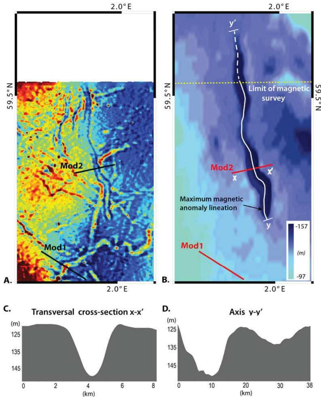
**Figure V-7.** 2D forward model profiles calculated for tunnel valleys. (a) vertical derivative magnetic map in order of 1.7; (b) bathymetry map (Weatherall et al., 2015) showing locations of 2D magnetic models, corresponding to a buried tunnel valley with no bathymetric expression (Mod1, Fig. V-8) and an underfilled tunnel valley (Mod2, Fig. V-9); Cross-sections (c) and (d) show bathymetric profiles perpendicular ( $x-x'$ ) and parallel ( $y-y'$ ) to the valley axis, respectively.
