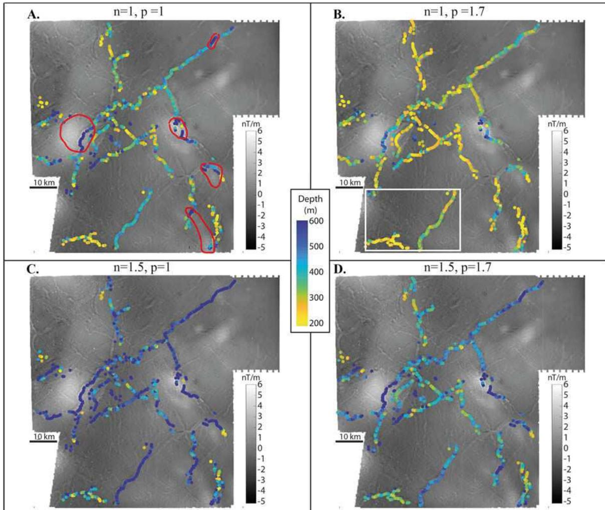
**Figure V-10.** Results of the depth estimation on the basis of the Euler deconvolution using complex algebra superimposed on the 1.7 order vertical derivative; Depth range is 200 to 600 m (100 m flight altitude is included within these values);  $n$ =structural index;  $p$ =derivative order; Euler' solution are calculated with: (a)  $n=1$  and  $p=1$ ; (b)  $n=1$  and  $p=1.7$ ; (c)  $n=1.5$  and  $p=1$ ; (d)  $n=1.5$  and  $p=1.7$
