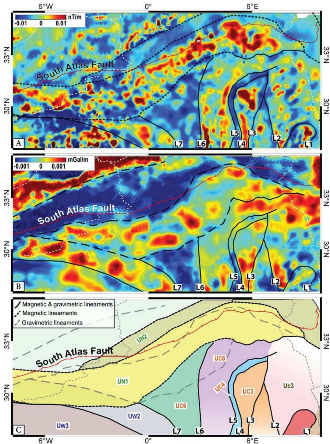
**Figure III-8:** Characterization of the Northern unit Set; (A) Vertical derivative applied to DRP of EMAG2 magnetic map; (B) Vertical derivative applied to Bouguer anomaly; (C) Synthetic map showing the distribution of superimposed magnetic and gravimetric boundaries discussed in the text (see Fig. III-10 for a full cover of the study area).
