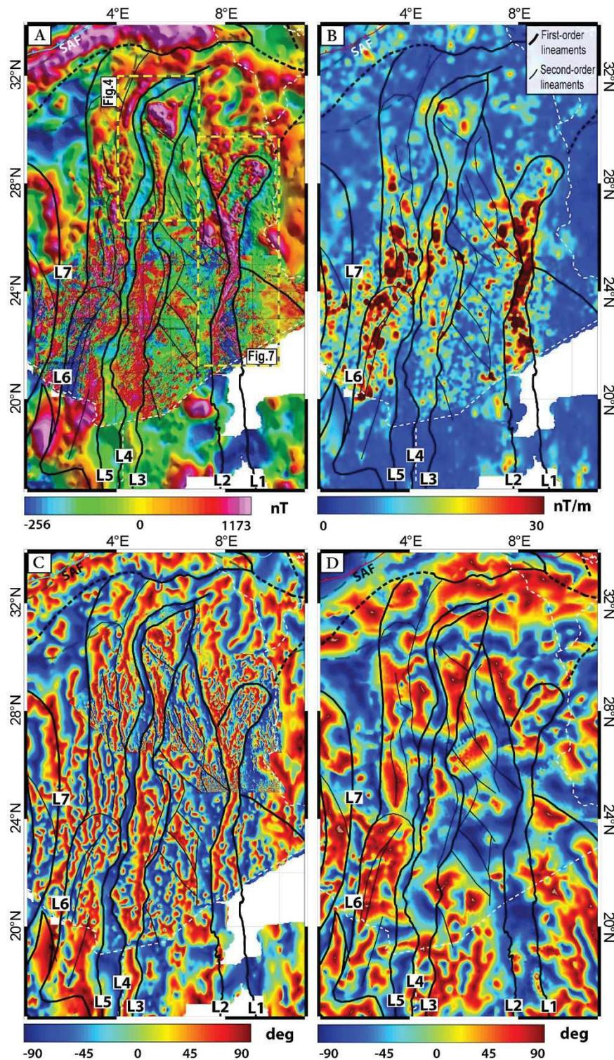
**Figure III-3:** Potential field data analysis of the Central unit set; (A) Double reduction to the pole (DRP) applied to the Total Magnetic Intensity map (TMI) compiled from the global aeromagnetic grid, aeromagnetic raster image of (Bournas et al., 2004) and EMAG2 grid; (B) Analytic signal magnetic map; (C) Tilt-depth after DRP using global aeromagnetic and EMAG2 magnetic maps; (D) Tilt-depth applied to Bouguer anomaly map. White dashed line: political boundaries.
