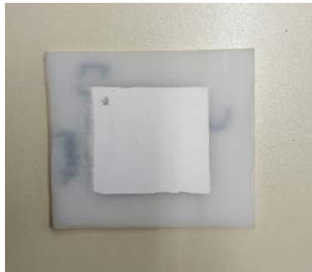
Figure 4.30 – TPT-coating over HDPE.
