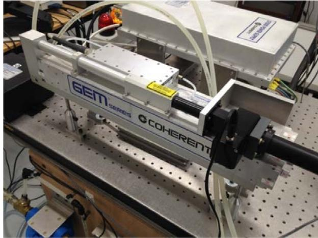
Figure 2.5 – Coherent GEM-100L CO<sub>2</sub> laser.
