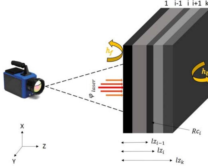
Figure 4.1 – Multi-layer material subjected to a short and non-uniform laser excitation at the front face, with a continuous measurement of the corresponding temperature recording via an IR camera.
