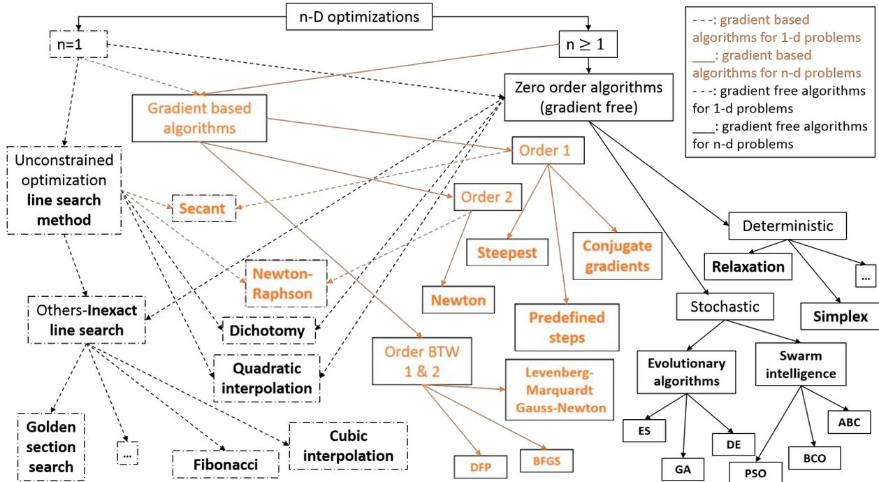
Figure 2.14 – The global classifications of commonly-used optimization methods.
