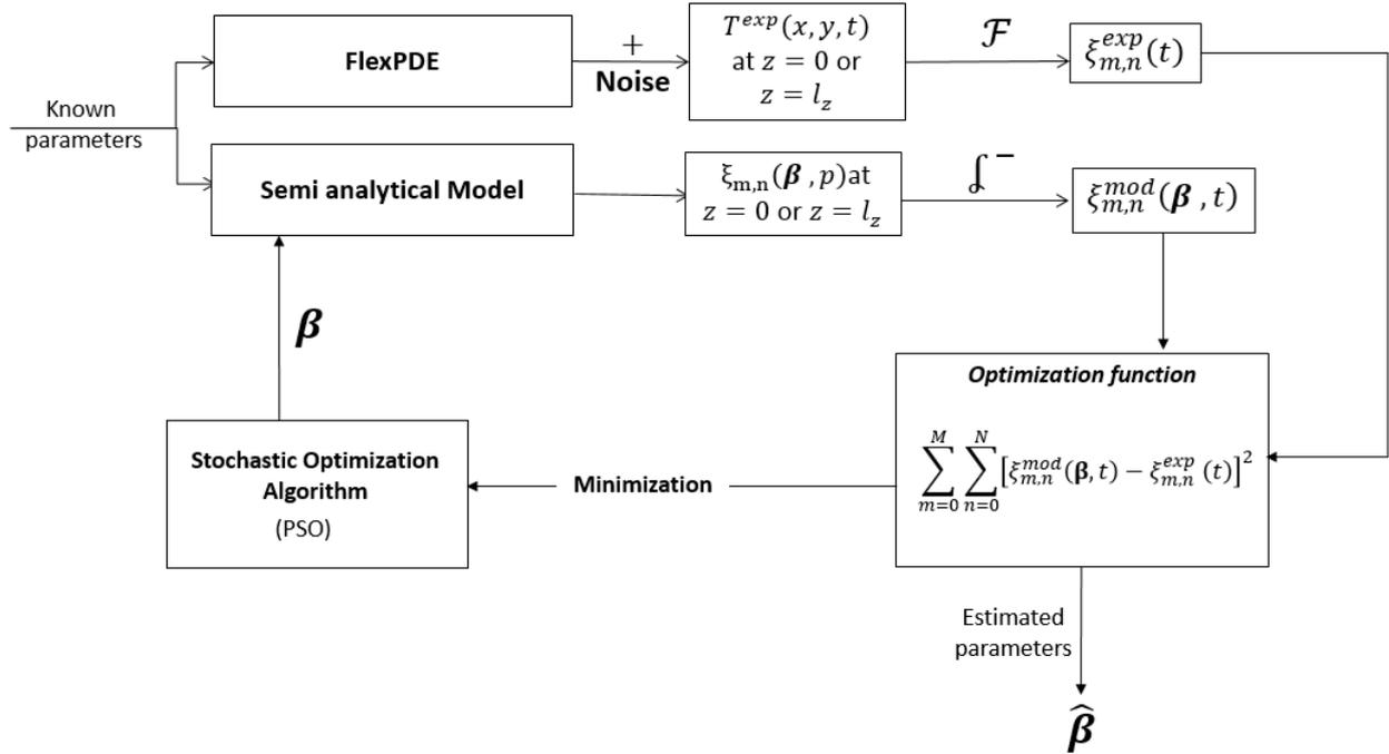
Figure 3.26 – General principle of the identification procedure consisting in finding the set of parameter  $\beta$  minimizing the differences between the synthetic projected data  $\xi^{exp}$  and the inverse projected model output  $\xi^{mod}$ .
