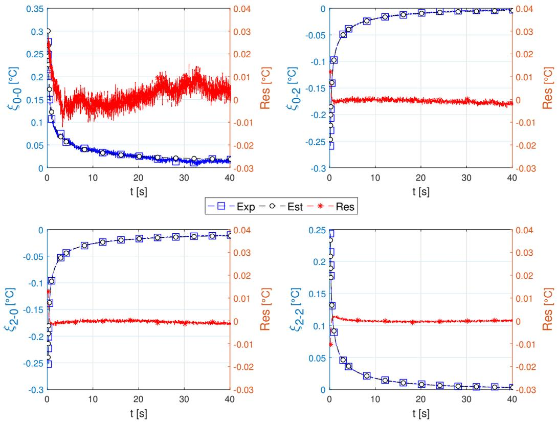
Figure 4.16 – Temporal evolution of the first four normalized harmonics concerning experimental (Exp.) and simulated data (Est.) using 6D estimation applied in config.(a). The absolute residue (Res) between both signals is plotted.
