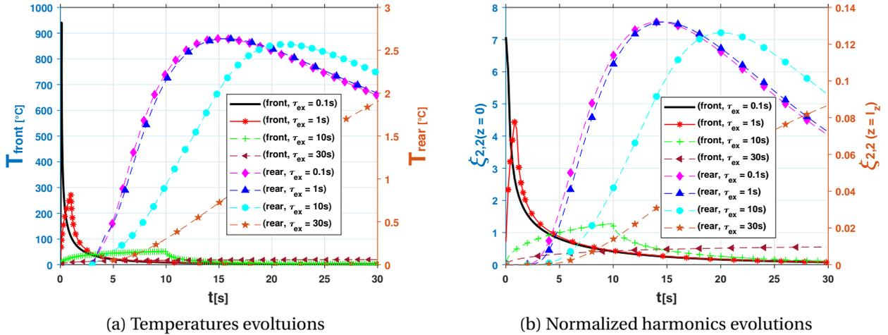
Figure 3.23 – Temperatures and normalized harmonics ( $m=n=2$ ) evolution at the front and rear for different pulse durations when applying an amount of energy  $Q=10\text{J}$ .
