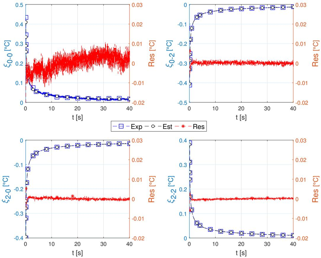
Figure 4.15 – Temporal evolution of the first four normalized harmonics concerning experimental (Exp.) and simulated data (Est.) using 4D estimation applied in config.(b). The absolute residue (Res) between both signals is plotted.
