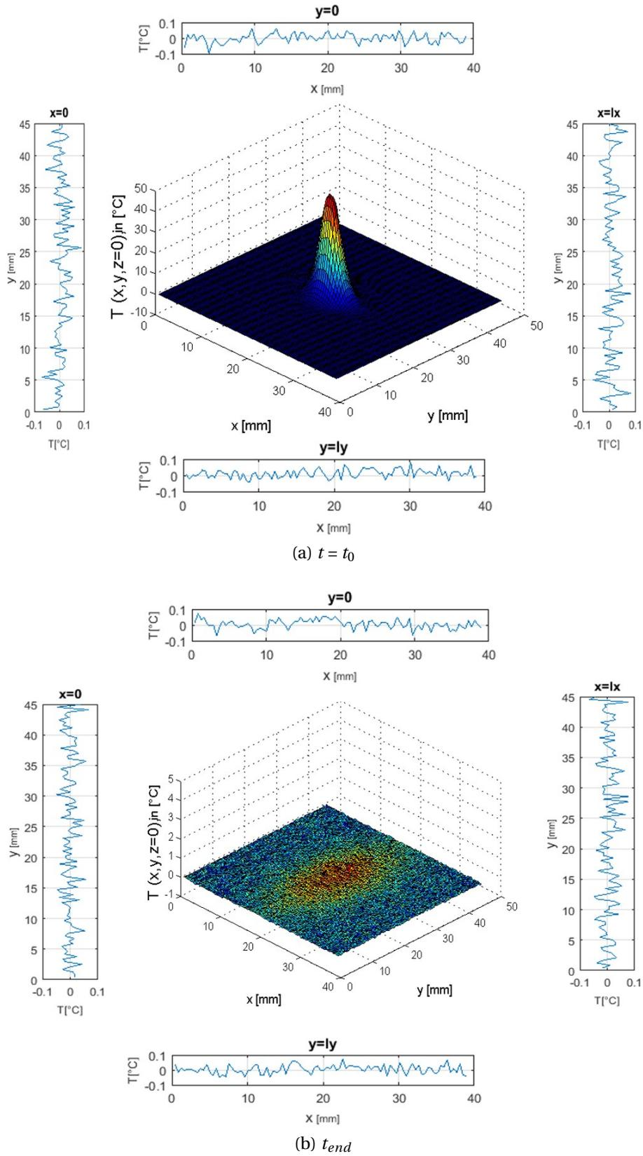
Figure 3.6 – Experimental temperature fields on the exposed surface ( $z = 0$ ), and temperature profiles at the boundaries ( $x = 0, x = l_x, y = 0$  and  $y = l_y$ ), just after the excitation and at the exploitation limit, for the orthotropic CFRP studied material.
