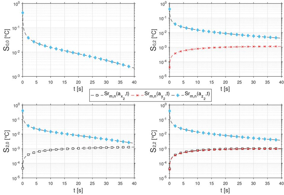
Figure 4.25 – Reduced sensitivities of the first 4 normalized harmonics to the composite diffusivities in config.(a).
