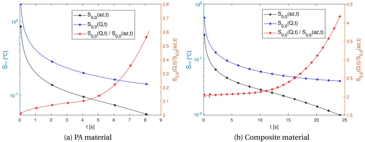
Figure 3.13 – Sensitivities of the front face first harmonics representing the mean fields  $\xi_{0,0}$ , to the in-depth diffusivities  $a_z$  and the total amount of heat  $Q$  absorbed at the surface of both samples, with their ratio in order to detect the decorrelation between both parameters.
