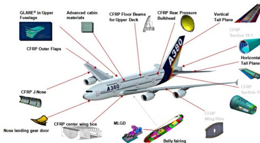
Figure 1.2 – CFRP application in airplanes [11].
