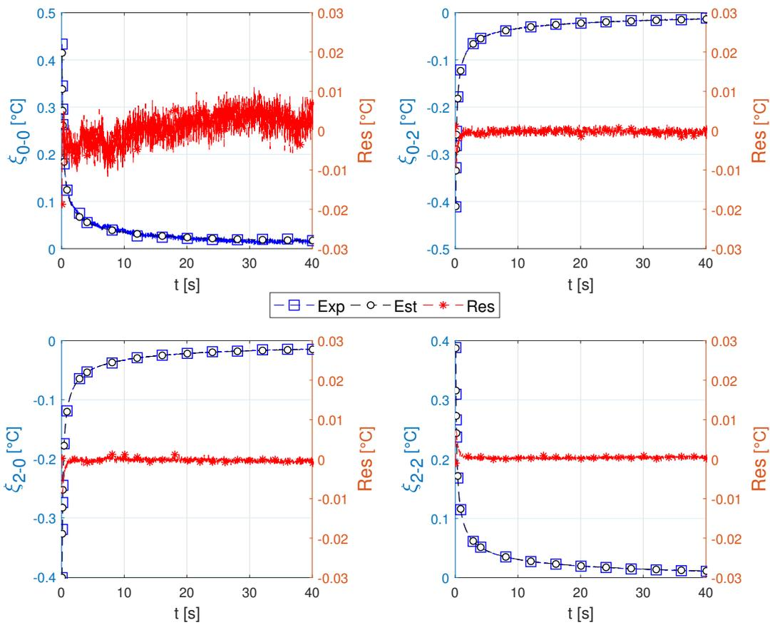
Figure 4.17 – Temporal evolution of the first four normalized harmonics concerning experimental (Exp.) and simulated data (Est.) using 6D estimation applied in config.(b). The absolute residue (Res) between both signals is plotted.
