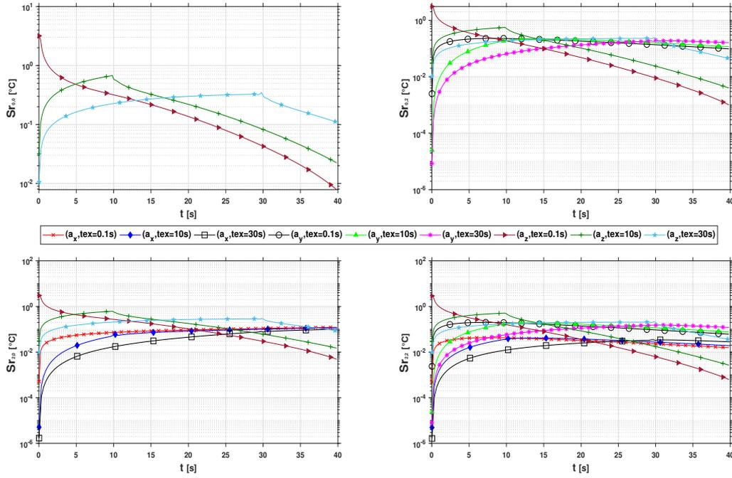
Figure 3.24 – Reduced sensitivities of the front first four even normalized harmonics to the composite diffusivities ( $a_x, a_y, a_z$ ), as a function of the laser pulse duration time (0.1, 10 and 30 s).
