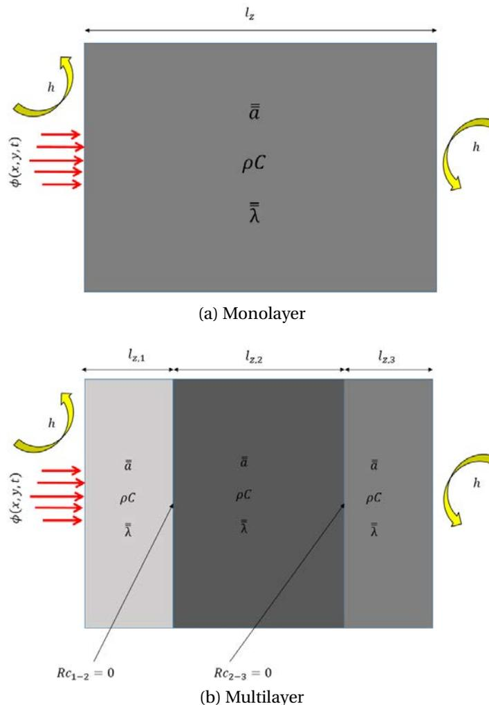
Figure 4.2 – Subdivision principle for the multilayers model validation.
