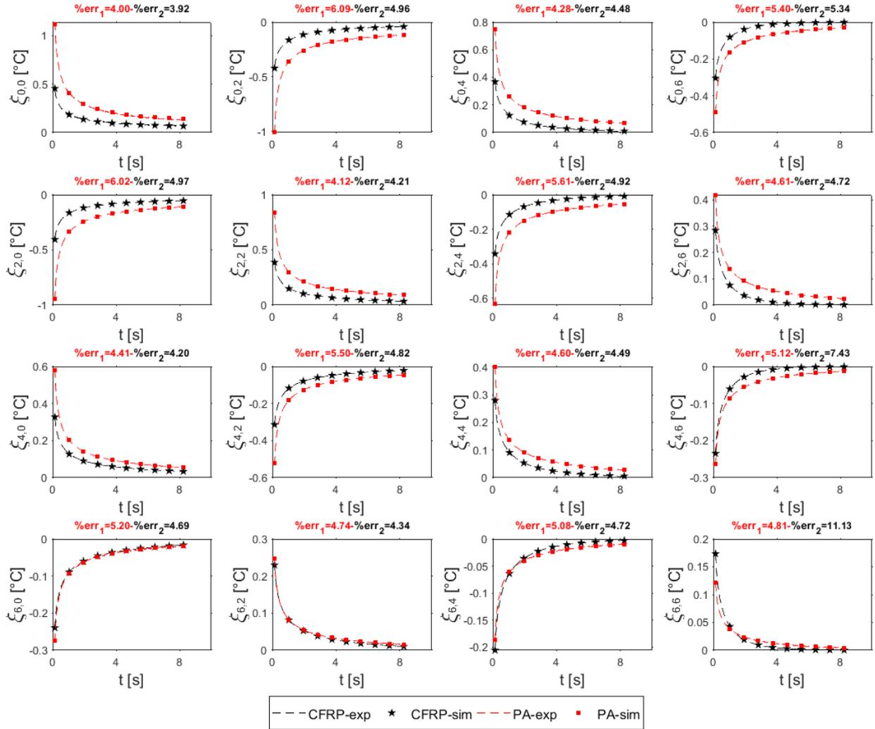
Figure 3.8 – Normalized harmonics temporal evolution for experimental (dotted or normal lines) and inversely estimated data (symbols), applied for the polyamide -PA (red; square) - and the composite -CFRP (black; pentagram) -samples.
