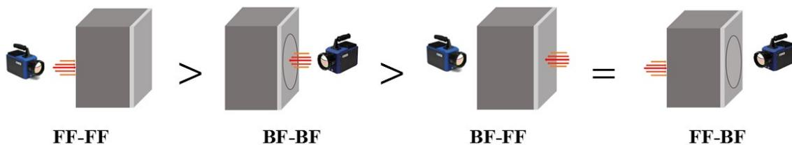
Figure 4.8 – The four possible configurations investigated for the search of the optimal estimation setup of the CFRP diffusivities. FF stands for “Front Face” and BF for “Back Face”. The first acronym corresponds to the excitation location, the second to the measurement.
