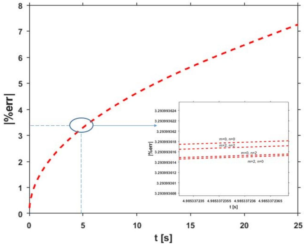
Figure 3.15 – Time evolution of the relative absolute deviation (error in %) between the front face normalized harmonics with an overall heat transfer  $h = 0 \text{ W} \cdot \text{m}^{-2} \cdot \text{K}^{-1}$  and those with  $h = 10 \text{ W} \cdot \text{m}^{-2} \cdot \text{K}^{-1}$ .
