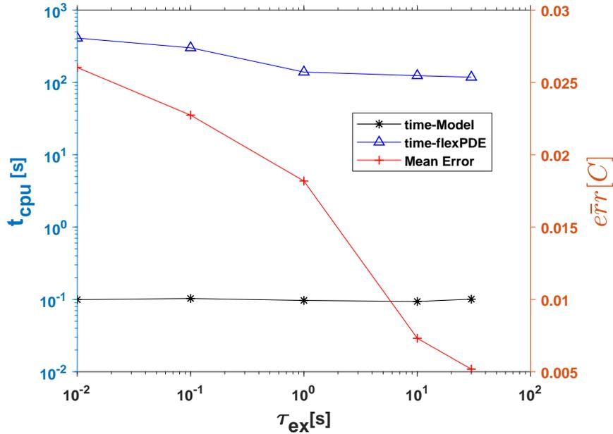
Figure 3.22 – Calculation time relative to both the pseudo-analytical and numerical simulations according to the excitation duration time  $\tau_{ex}$ , with the average quadratic error between the two signals.
