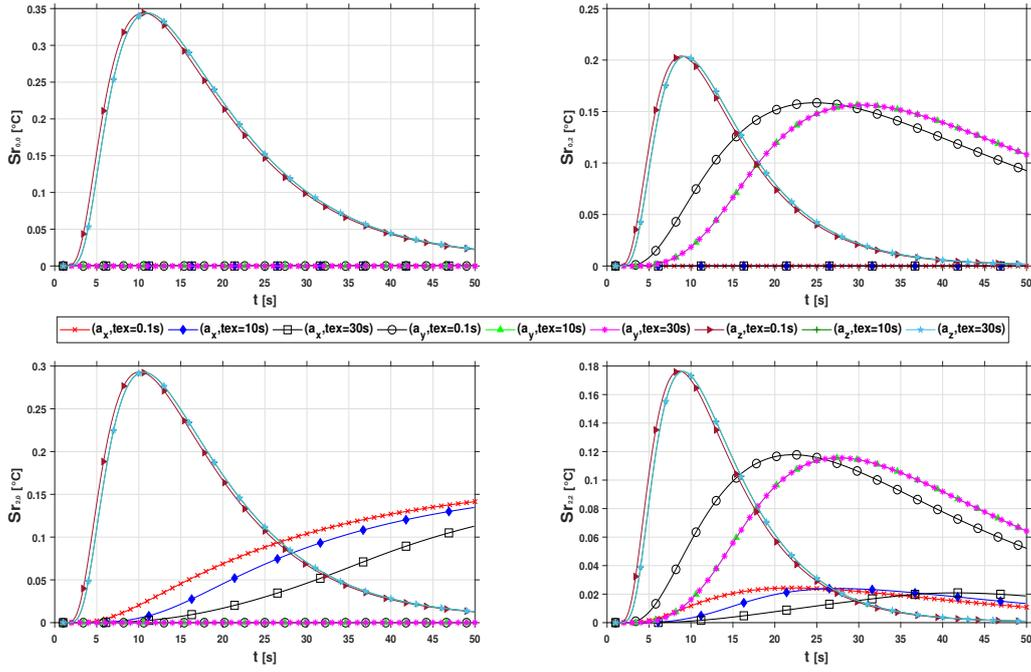
Figure 3.25 – Reduced sensitivities of the rear first four even normalized harmonics to the composite diffusivities ( $a_x, a_y, a_z$ ), as a function of the laser pulse duration time (0.1, 10 and 30 s).
