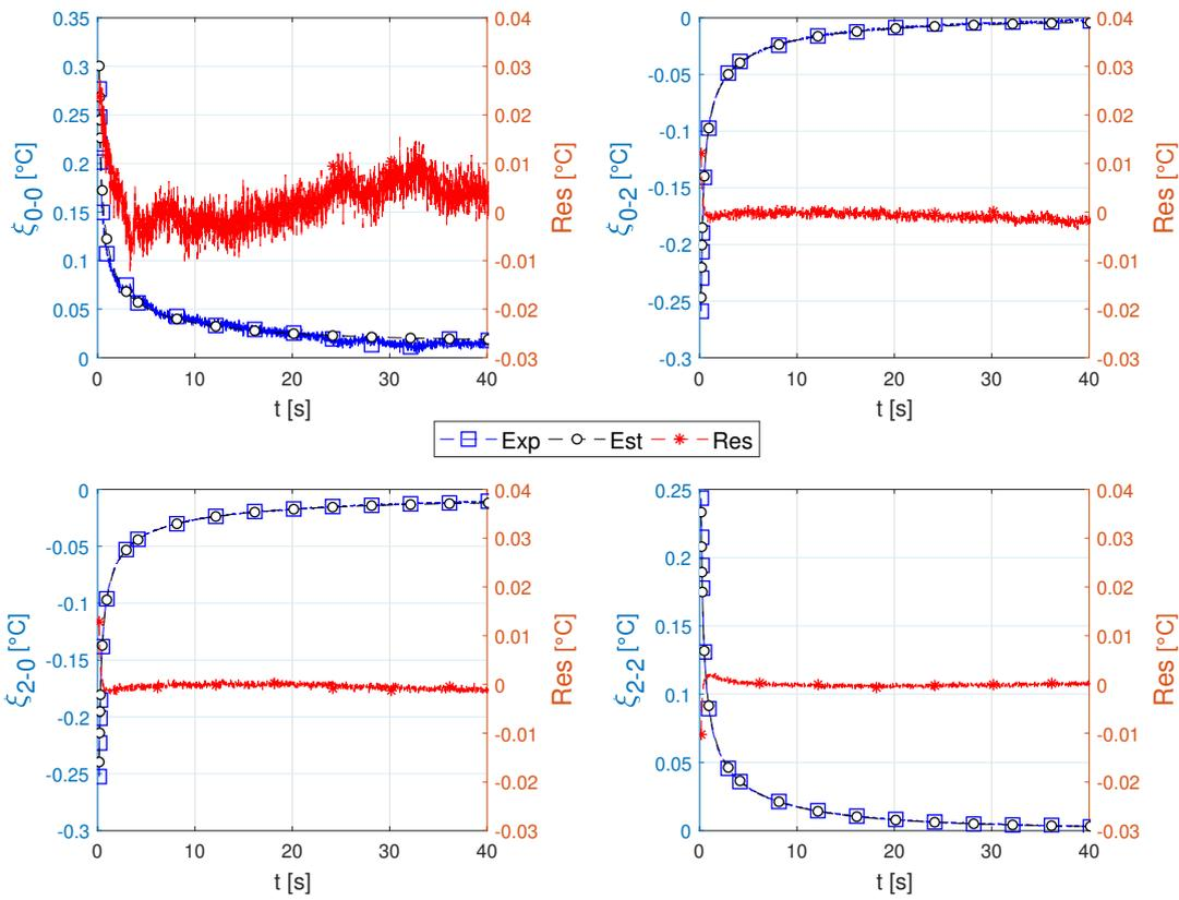
Figure 4.14 – Temporal evolution of the first four normalized harmonics concerning experimental (Exp.) and simulated data (Est.) using 4D estimation applied in config.(a). The absolute residue (Res) between both signals is plotted.
