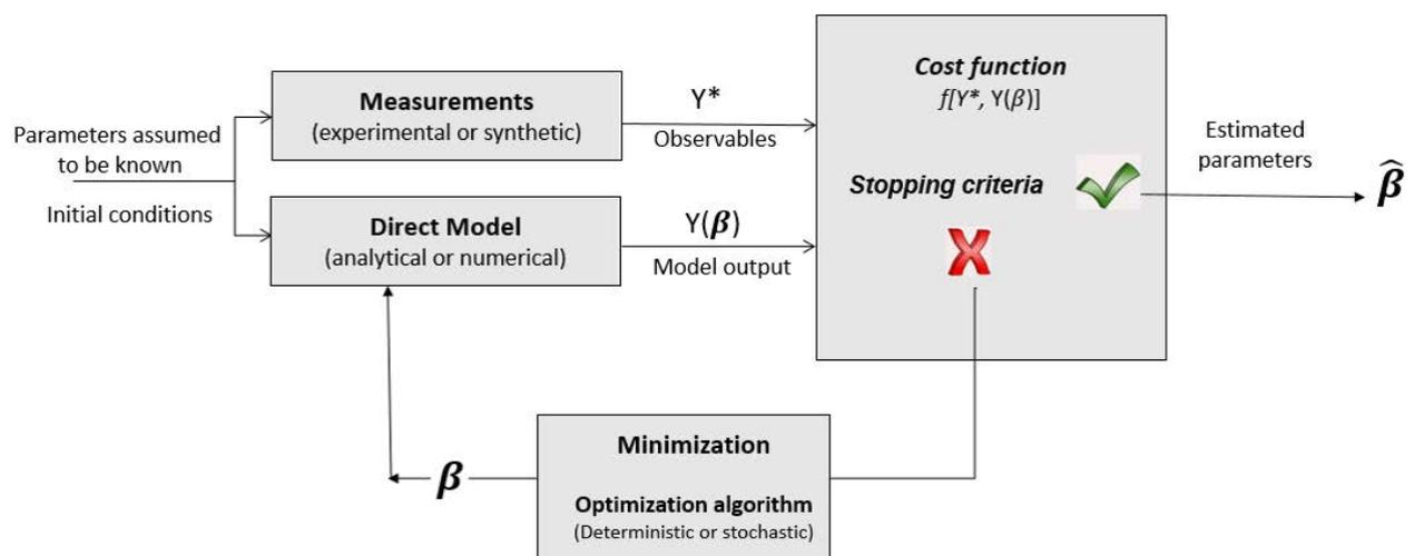
Figure 2.1 – Inverse problem principle and main sections (steps).
