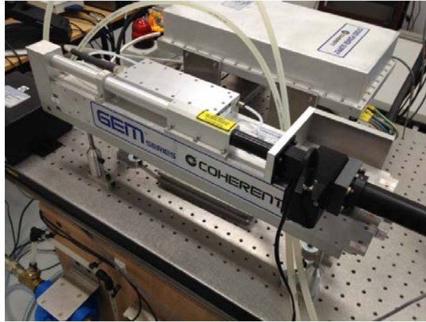
Figure 2.5 – Coherent GEM-100L CO 2 laser.
