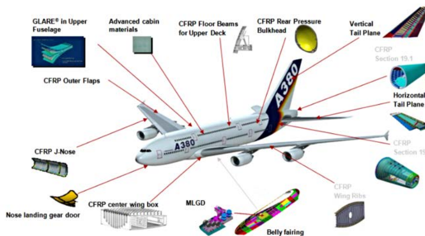
Figure 1.2 – CFRP application in airplanes [11].
