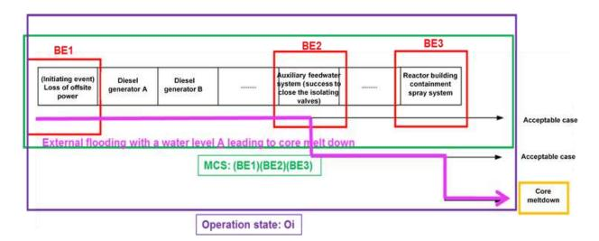
Figure 3.6 Illustration of a MCS in an individual reduced-order model
