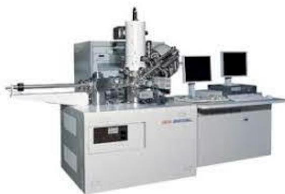
**Figure 2-14 : Microscope Auger JEOL JAMP 9500F**
