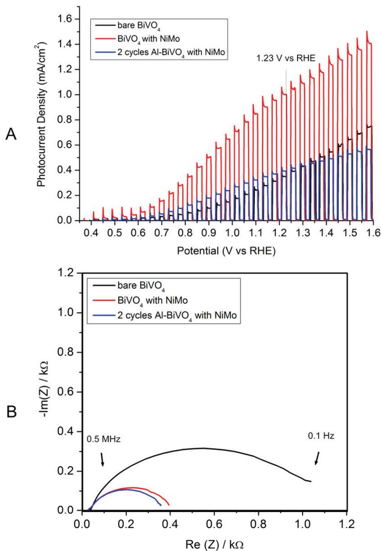
Figure 27. (A) LSV (electrolyte: 0.1 M Na-Pi pH 7, scan rate: 10 mV/s) and (B) Nyquist plots for bare BiVO<sub>4</sub>, BiVO<sub>4</sub> with NiMo and 2 cycles Al-BiVO<sub>4</sub> with NiMo
