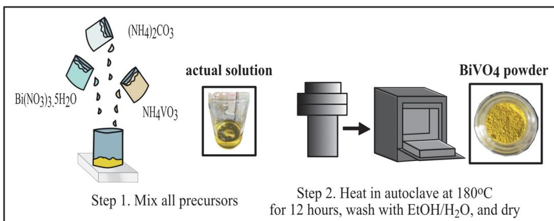
Figure 16. Hydrothermal synthesis of BiVO<sub>4</sub> powder
