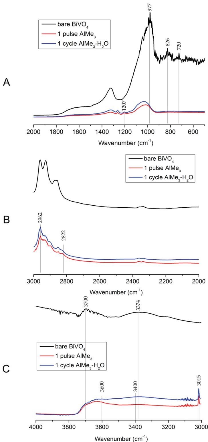
Figure 21. FTIR Spectra of dehydroxylated bare  $\text{BiVO}_4$  powder,  $\text{BiVO}_4$  powder with 1 pulse of  $\text{AlMe}_3$  and 1 cycle  $\text{AlMe}_3\text{-H}_2\text{O}$  at (A) 2000-500  $\text{cm}^{-1}$  wavenumbers, (B) 3000-2000  $\text{cm}^{-1}$  wavenumber, (C) 4000-3000  $\text{cm}^{-1}$  wavenumber
