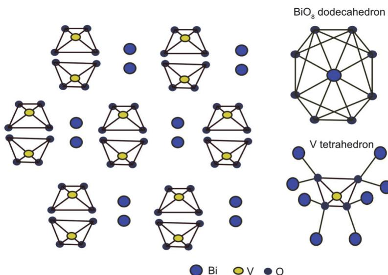
Figure 2. BiVO<sub>4</sub> monoclinic scheelite structure
