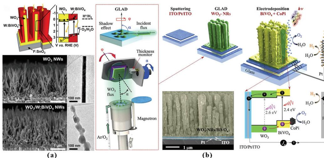
Figure 4. (a)  $\text{WO}_3/\text{BiVO}_4$  core-shell nanowires (NWs) according to Rao *et al*<sup>104</sup> and (b)  $\text{WO}_3/\text{BiVO}_4$  core-shell nanorods (NRs) by Pihosh *et al*<sup>57</sup>. Image (a) reprinted/adapted with permission from<sup>104</sup>, Copyright American Chemical Society, 2014. Image (b) used under the Creative Commons CC-BY license attributed to<sup>57</sup>. Copyright Nature Publishing Group, 2015.
