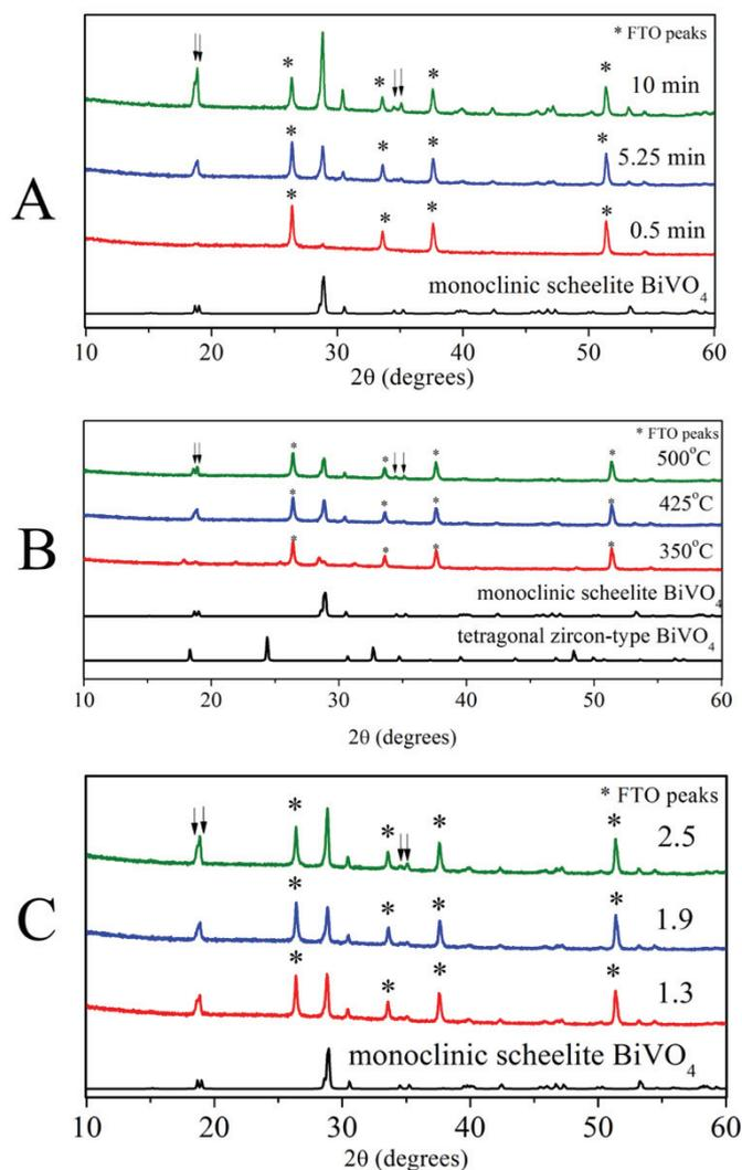
Figure 8. XRD spectra of the bare  $\text{BiVO}_4$  photoanodes synthesized at different: (a) electrodeposition times, (b) calcination temperatures, and (c) Bi-KI to Benzoquinone-EtOH ratio, as specified in Table 4.
