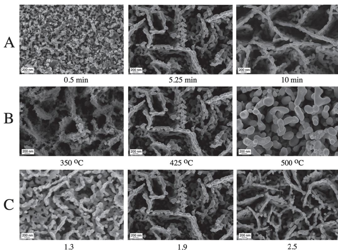
Figure 7. FESEM images of the bare BiVO<sub>4</sub> photoanodes synthesized at different: (A) electrodeposition times, (B) calcination temperatures, and (C) Bi-KI to Benzoquinone-EtOH ratio, as detailed in Table 4.
