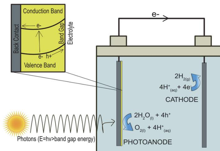
Figure 1. Schematic diagram of photoelectrochemical water splitting
