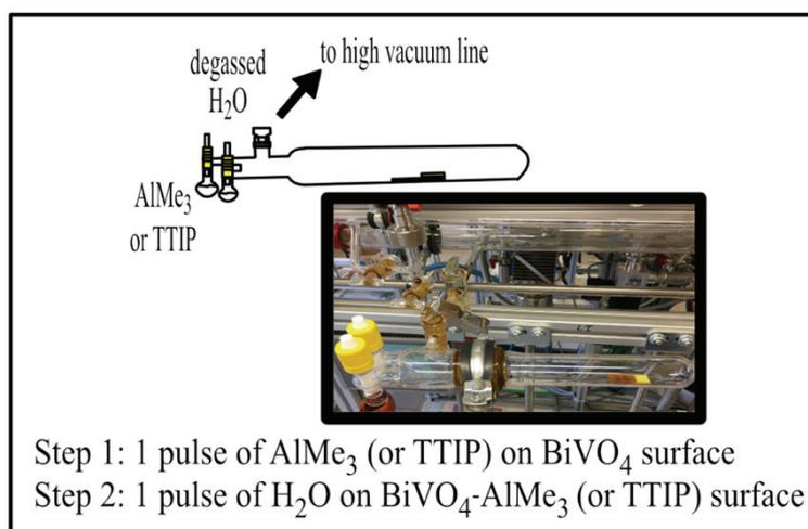
Figure 20. Surface modification of BiVO<sub>4</sub> electrode
