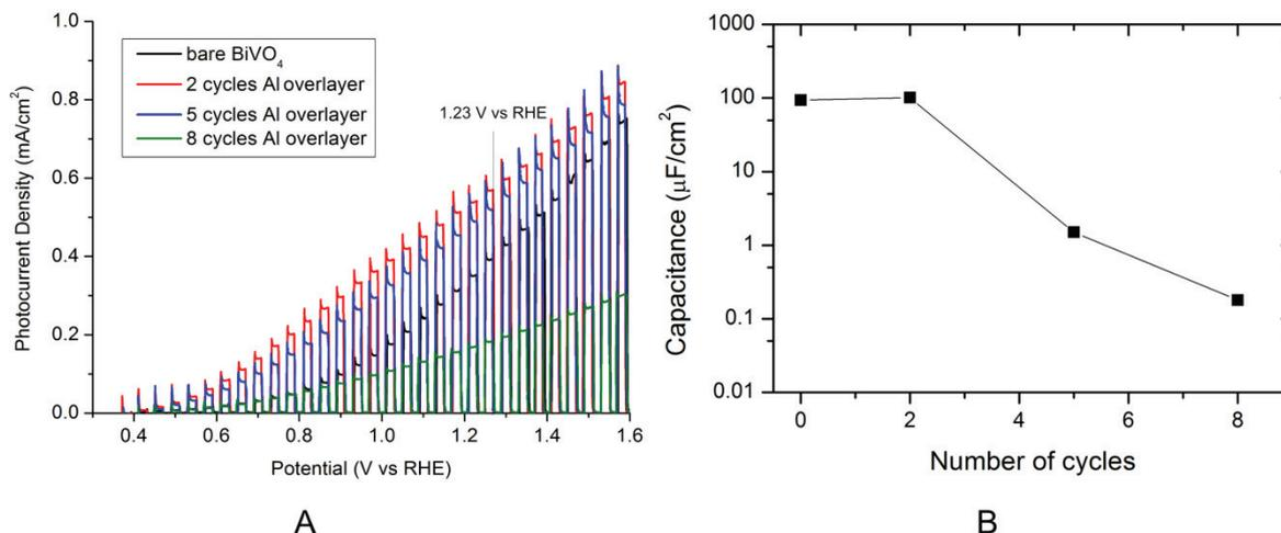
Figure S2. (A) Linear sweep voltammograms of bare BiVO<sub>4</sub> and Al-modified BiVO<sub>4</sub> (electrolyte: 0.1M Na-Pi pH 7, scan rate: 10 mV/s) and (B) Surface capacitance measurements at various cycles
