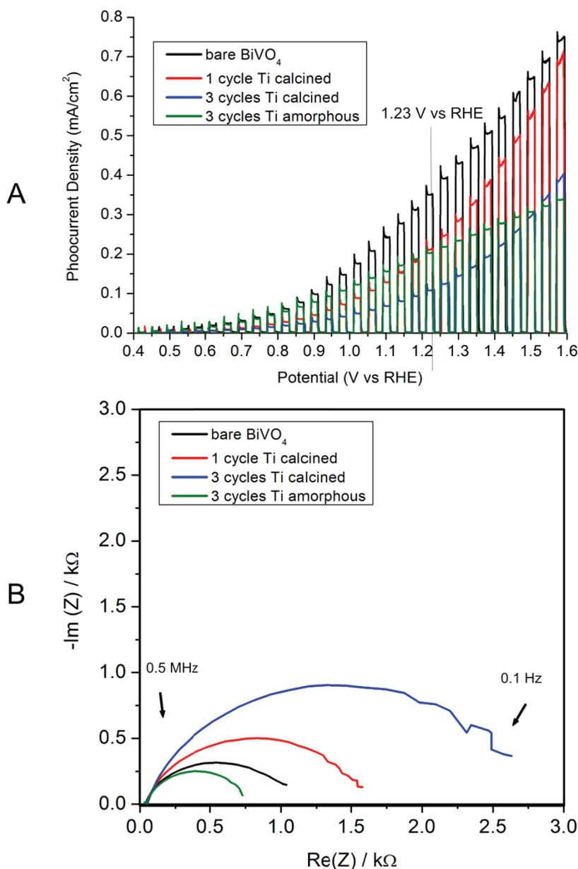
Figure 26. (A) LSV (electrolyte: 0.1 M Na-Pi pH 7, scan rate: 10 mV/s) and (B) Nyquist impedance plots for bare and Ti-modified BiVO<sub>4</sub>
