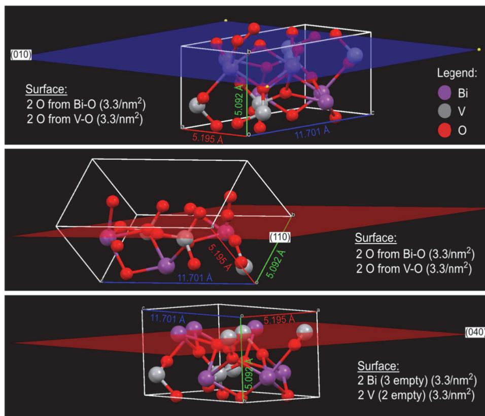
Figure A10. BiVO<sub>4</sub> surface termination considering (010), (110), and (040) surfaces
