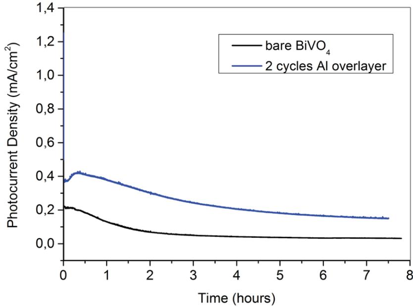
Figure 25. Stability test (chronoamperometry) plot for 2 cycles Al and bare BiVO<sub>4</sub> (electrolyte: 0.1 M Na-Pi pH 7, potential: 1.23 V vs RHE)
