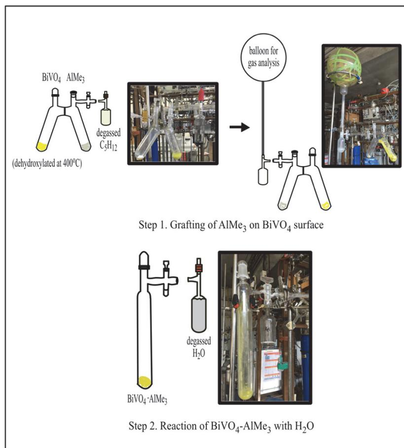
Figure 19. Surface modification of  $\text{BiVO}_4$  powder with Al
