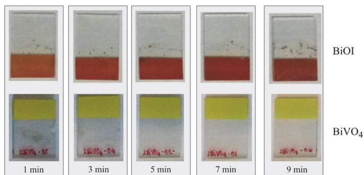
Figure A2. Electrodeposited BiOI (TOP) and synthesized BiVO<sub>4</sub> (BOTTOM) at different electrodeposition times, (Bi-KI to benzoquinone-ethanol ratio at 2.5 and the calcination temperature of 450°C)
