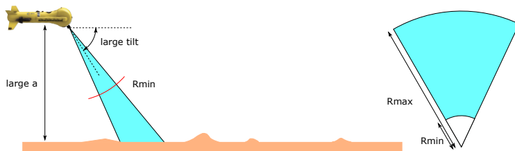
Figure 2.12: Small coverage area with an high altitude and a large tilt angle.
