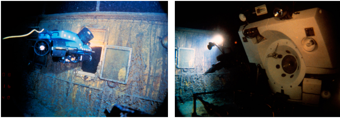
Figure 1.5: Robots used for the exploration of the RMS Titanic wreck which sank in 1912. On the left, the unmanned ROV Jason Jr. taking some photographs, tethered by the manned submersible Alvin on the right picture.
