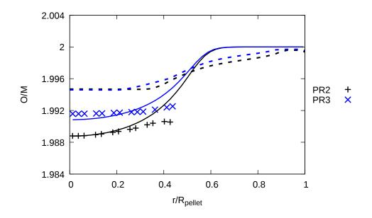
Figure 4.32: Initial O/M (dashed lines), steady-state O/M calculated with OXIRED (solid lines) compared to the O/M calculated with ANGE (points). PR2 is in black and PR3 in blue.
