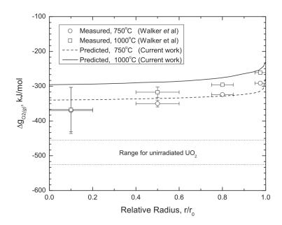
Figure 2.40: Comparison of the oxygen potential calculated by Piro et al. [12] with experimental data from Walker et al. [7].
