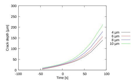
Figure 5.55: Cladding crack depth calculated at the triple point during PR5 with different initial crack depths.
