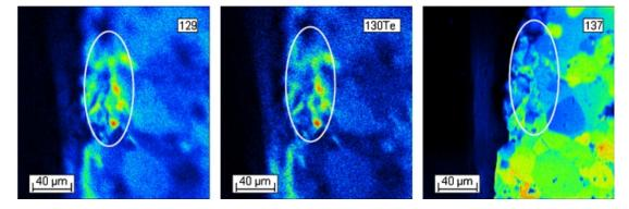
Figure 2.12: SIMS images presenting <sup>129</sup>I, <sup>130</sup>Te and <sup>137</sup>Cs near the pellet periphery. Dark blue corresponds to the lowest concentration and red to the highest concentration [61].
