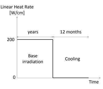
Figure 3.1: Schematic representation of the power sequence used in the simulation of iodine isotopic evolution.
