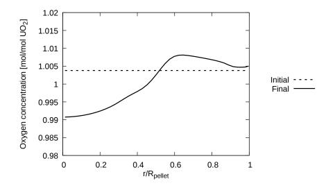
Figure 5.8: Radial profile of total oxygen content calculated at the end of the holding period of PR2 (solid curve) and the initial oxygen concentration (dashed curve).
