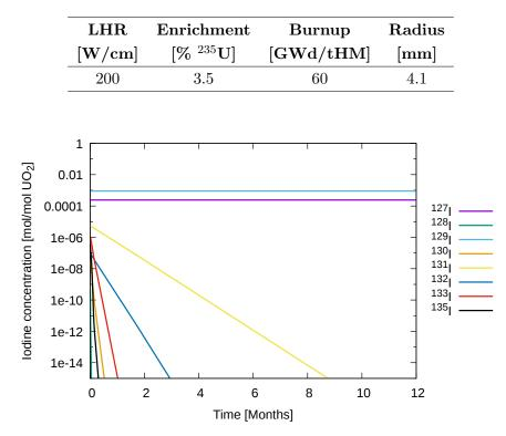
Figure 3.2: Concentrations of iodine isotopes calculated in PRODHEL plotted as a function of time at zero power. The plot starts at the end of base irradiation. Simulation parameters are given in Table 3.3.
