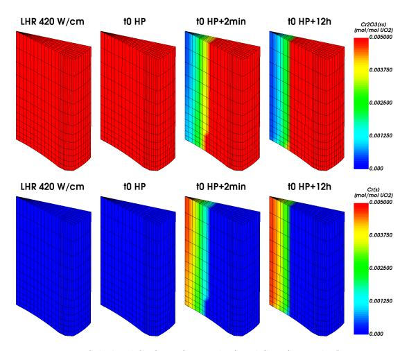
Figure 5.21: Calculated  $Cr_2O_{3(ss)}$  (upper plots) and  $Cr_{(s)}$  (lower plots) concentrations [mol/mol UO<sub>2</sub>] at different times during power ramp PR2.
