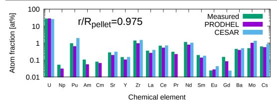
Figure 3.16: PRODHEL calculations of the local atom fractions of chemical elements compared to EPMA measurements from Walker et al. [7] and to CESAR calculations at  $r/R_{pellet}=0.975$ .
