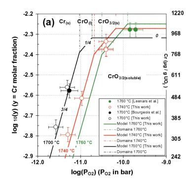
Figure 2.9: Relation between chromium mole fraction in UO<sub>2</sub> (i.e., chromium solubility) and oxygen partial pressure for various temperatures. One may notice the stability areas for  $Cr_{(s)}$ ,  $CrO_{(l)}$  and  $CrO_{3/2(s)}$ . Figure adapted from [53]. Experimental data from [53–55].
