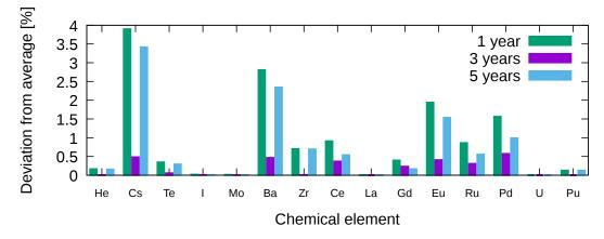
Figure 3.9: Deviations from average value in PRODHEL calculations of the integral weight fractions of chemical elements after 1, 3 or 5 years of cooling.
