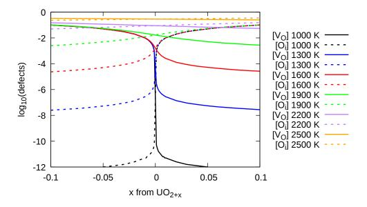
Figure 4.34: Frenkel defects concentration  $UO_{2\pm x}$  calculated from Gibbs energy of formation of Frenkel defects. Adapted from Berthinier et al. [91]. Solid lines correspond to vacancies and dashed lines to interstitial atoms.
