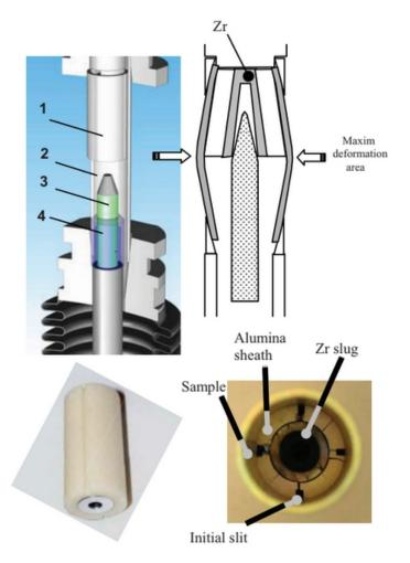
Figure 2.32: "Expanding mandrel sample configuration for I-SCC investigations of irradiated fuel cladding materials, the aluminia insert with 4 longitudinal slits and the pure Zr mandrel in the central part and a cross section of a cladding sample after mandrel testing [127]; 1–alumina sheath; 2–Zircaloy cladding (sample); 3–plunger; 4–channel from pure Zr" [128].
