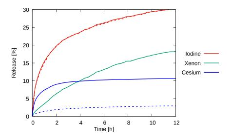
Figure 5.30: Calculated release of Cs, I and Xe during power ramp PR2. Solid lines refer to the simulation with oxygen transport, dashed lines refer to the simulation without oxygen transport (t=0 corresponds the beginning of the holding period, "t0").
