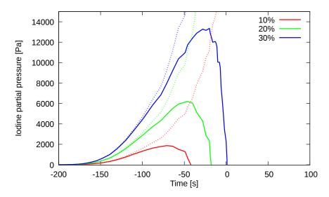
Figure 5.57: Solid lines correspond to the iodine partial pressure taking into account interactions of the "reactive" iodine with the free cesium and radiolysis of CsI. Dotted lines correspond to the iodine partial pressure of the 'reactive' iodine and radiolysis of CsI. Different colors correspond to different fractions of CsI that undergo decomposition by radiolysis.
