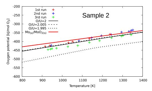
Figure 3.37: Calculated oxygen potential compared to experimental measurements from Matzke [67]. Burnup 34.5 GWd/tHM. O/U refers to the initial composition.
