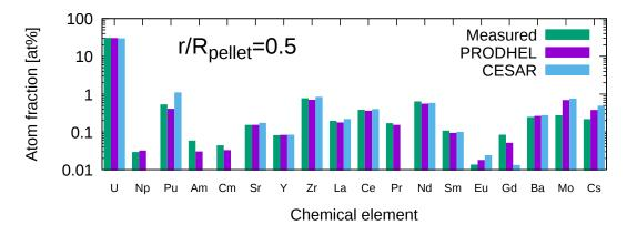
Figure 3.14: RODHEL calculations of the local atom fractions of chemical elements compared to EPMA measurements from Walker et al. [7] and to CESAR calculations at  $r/R_{pellet}=0.5$ .
