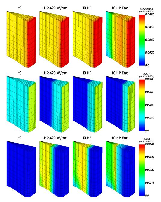
Figure 5.44: Concentrations [mol/mol UO<sub>2</sub>] of  $Cs_2MoO_{4(s,l)}$  (top),  $CsI_{(s,l)}$  (middle) and  $CsI_{(q)}$  at different moments of PR5.
