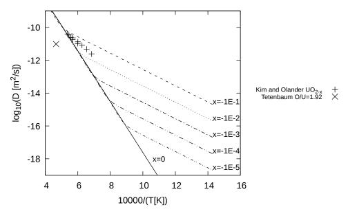
Figure 4.38: Self-diffusion coefficient based on the work of Berthinier [91] compared to experimental data [88,94]. Hypostoichiometric domain.
