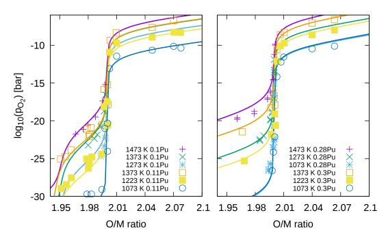
Figure 3.21: Calculated oxygen partial pressure in  $U_{1-y}Pu_yO_{2\pm x}$  (lines) as a function of O/M, temperature and Pu mole fraction compared to measured values (symbols). Experimental data from [168–170].
