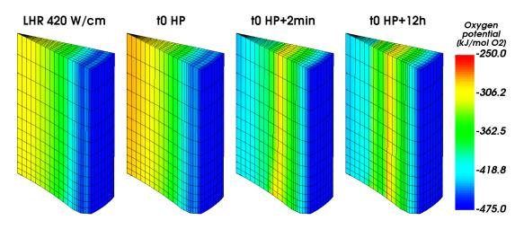
Figure 5.18: Calculated oxygen potentials  $[kJ/mol O_2]$  in the fuel fragment at different times during power ramp PR2.
