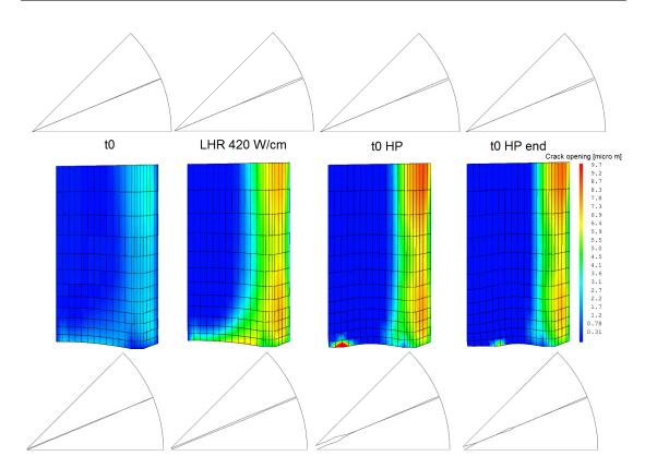
Figure 5.50: Calculated pellet radial crack opening at different times during PR5. Upper graphs give the mid-pellet plane. Lower graphs the inter-pellet plane. Isovalues give the distribution of crack opening on the fracture surface.
