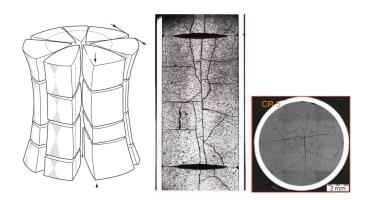
Figure 1.9: Hour-glassing of a fuel pellet [3].
