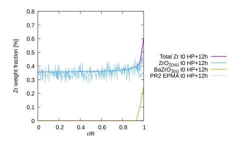
Figure 5.24: Calculated  $ZrO_{2(ss)}$  and  $BaZrO_{3(s)}$  concentrations compared to the EPMA measurement of Zr weight fraction after power ramp PR2.
