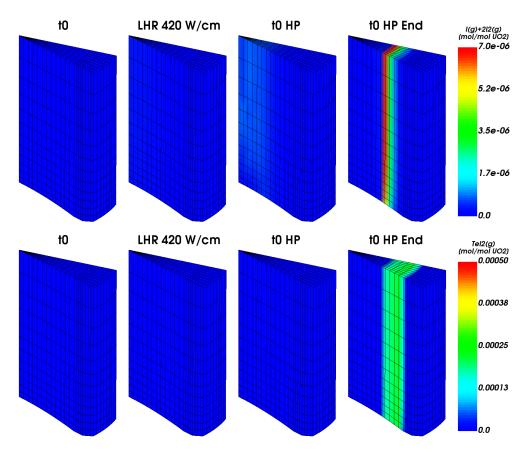
Figure 5.42: Concentration [mol/mol UO<sub>2</sub>] of  $I_{(g)}+2I_{2(g)}$  (upper figures) and  $TeI_{2(g)}$  (lower figures) at different moments of PR5.
