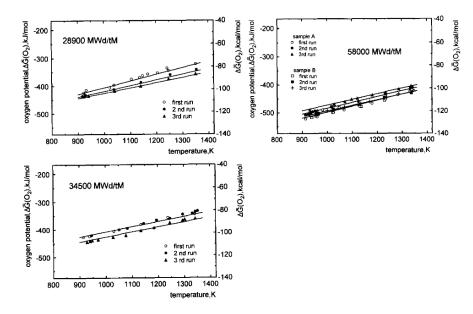
Figure 2.16: Oxygen potential measurements of samples with burnups of 28.9 GWd/tHM (top left), 34.5 GWd/tHM (bottom left) and 58 GWd/tHM (top right). Adapted from [67].
