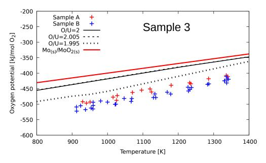
Figure 3.38: Calculated oxygen potential compared to experimental measurements from Matzke [67]. Burnup 58 GWd/tHM. O/U refers to the initial composition.
