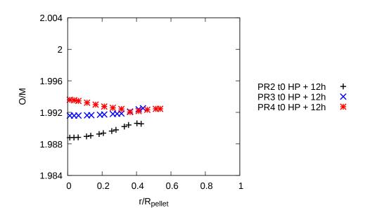
Figure 4.31: O/M radial profiles from ANGE calculations.
