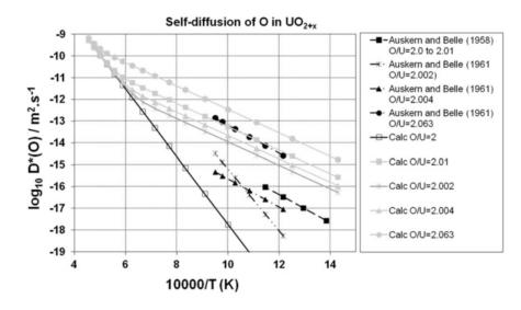
Figure 2.23: Figure from Berthinier et al. [91]. Comparison of the self-diffusion coefficient of oxygen proposed by the author with the experimental data [92,93]. Values for the hyperstoichiometric domain.
