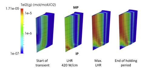
Figure 2.44:  $\operatorname{TeI}_{2(g)}$  at different times during the power ramp simulated by Baurens et al. [14].
