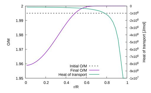
Figure 4.4: Example of OXIRED calculations with a nonlinear heat of transport.
