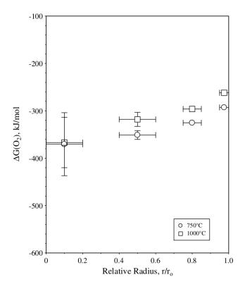
Figure 2.18: Comparison of oxygen potentials at different temperatures [7].
