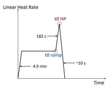
Figure 3.5: Schematic representation of PR1. The conditioning period lasts until "t0 ramp". The maximum LHR is reached at "t0 HP". Durations of power transients are marked.
