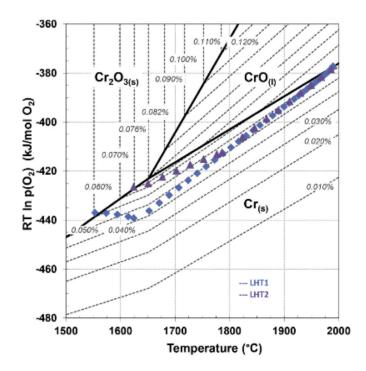
Figure 3.27: Phase stability diagram of chromium in  $UO_2$ . The dashed curves are the chromium iso-solubility curves. The labels in italics are the iso-solubility expressed in %wt Cr. The blue and purple points refer to the power ramps studied by Riglet-Martial [52].
