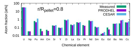
Figure 3.15: PRODHEL calculations of the local atom fractions of chemical elements compared to EPMA measurements from Walker et al. [7] and to CESAR calculations at  $r/R_{pellet}=0.8$ .
