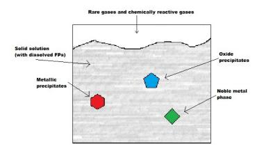
Figure 2.1: Schematic of irradiated fuel.
