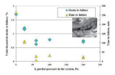
Figure 2.33: Total diametral strain to failure (blue points) and time to failure (yellow points) as a function of  $I_2$  partial pressure. Figure from [128].
