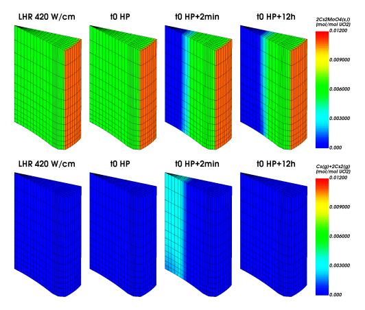
Figure 5.28: Calculated  $2Cs_2MoO_{4(s,l)}$  and  $Cs_{(g)}+2Cs_{2(g)}$  concentrations in the fuel fragment at different times during power ramp PR2.
