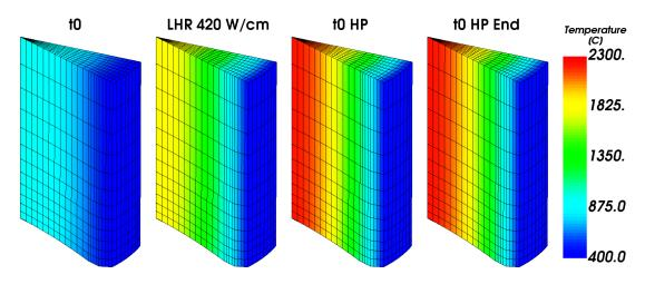
Figure 5.32: Temperature [°C] calculated at different times during PR5.
