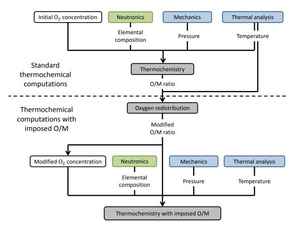
Figure 5.2: Schematic representation of thermochemical calculations with (bottom part) and without (top part) imposing the O/M ratio. Colors of boxes are consistent with Figure 5.1.
