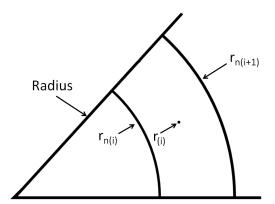
Figure 4.1: Visualization of the 1D discretization used in the OXIRED model.
