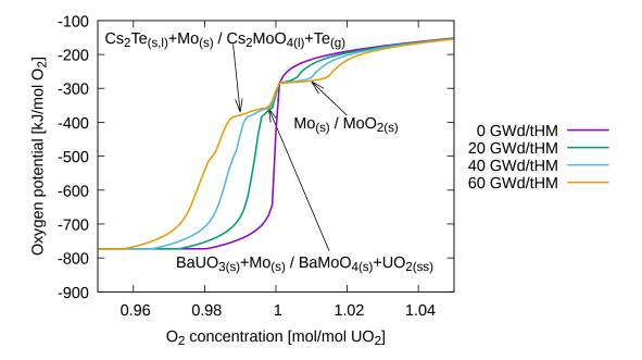
Figure 3.32: The oxygen potential at 1500  $^{\circ}$ C at different burnups as a function of the total oxygen concentration. Elemental compositions used in calculations are given in Table 3.17.
