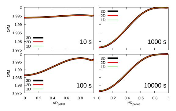
Figure 4.11: 1D, 2D and 3D O/M radial profiles at different times.
