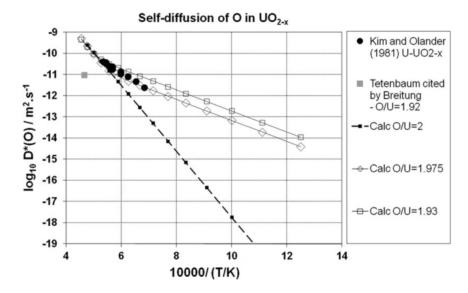
Figure 2.24: Figure from Berthinier et al. [91]. Comparison of the self-diffusion coefficient of oxygen proposed by the author with the experimental data [88,94]. Values for the hypostoichiometric domain.
