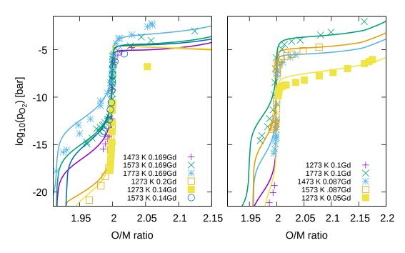
Figure 3.22: Calculated oxygen partial pressure in  $U_{1-y}Gd_yO_{2\pm x}$  (lines) as a function of O/M, temperature and Gd mole fraction compared to measured values (symbols). Experimental data from [171–173].
