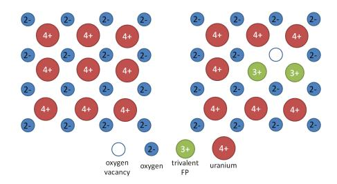
Figure 3.30: Schematic representation of  $UO_2$  lattice when a trivalent FP replaces a U atom after fission (adapted from Olander [181], chapter 12, Figure 12.8). Left figure: perfect  $UO_2$  lattice. Right figure: irradiated fuel.
