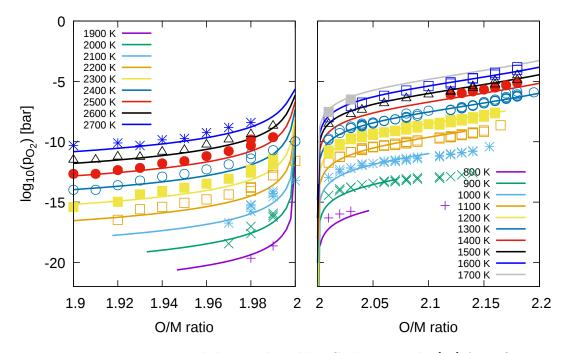
Figure 3.20: Experimental data gathered by Guéneau et al. [40] for  $UO_{2\pm x}$  (symbols) compared to ANGE calculations (lines) using the optimized Lindemer and Besmann model.
