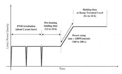
Figure 1.17: Schematic illustration of a power ramp test [24].
