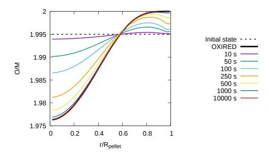
Figure 4.5: O/M radial profiles calculated with OXIRED (thick black curve) and OXITRAN at different times.
