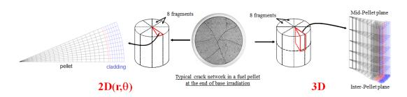
Figure 4.8: Examples of 2D and 3D meshes used in Cast3M.
