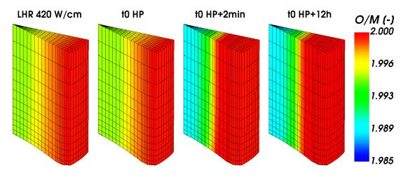
Figure 5.16: Calculated O/M ratios [-] in the fuel fragment at different times during the power ramp PR2.
