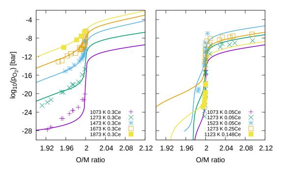
Figure 3.24: Calculated oxygen partial pressure in  $U_{1-y}Ce_yO_{2\pm x}$  (lines) as a function of O/M, temperature and Ce mole fraction compared to measured values (symbols). Experimental data from [177–179].
