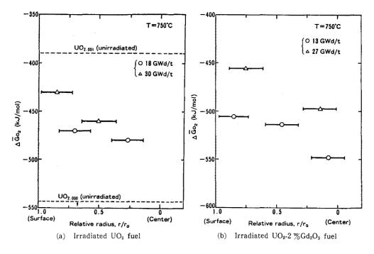
Figure 2.15: Oxygen potential measured in irradiated  $UO_2$  (a) and gadoliniumdoped fuel (b). Adapted from [65].
