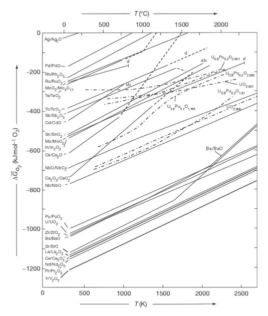
Figure 2.2: Relative partial molar Gibbs free energies of oxygen of the fission product oxides and of  $UO_{2+x}$  [19].
