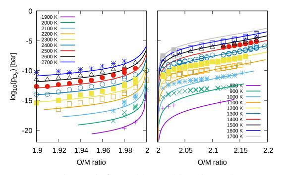
Figure 3.19: The original  $UO_{2\pm x}$  model proposed by Lindemer and Besmann [166] (lines) compared to the experimental data gathered by Guéneau et al. [40] (symbols).
