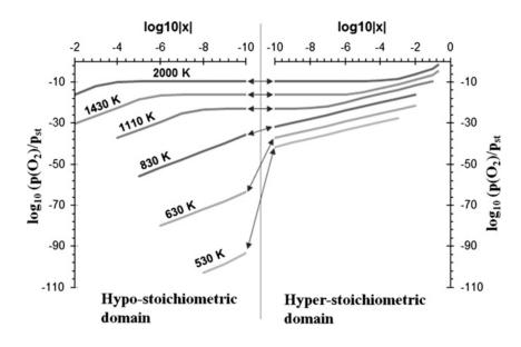
Figure 2.26: Oxygen partial pressure as a function of the logarithm of the stoichiometry deviation. Different curves correspond to different temperatures. Calculations done by Berthinier et al. [91].
