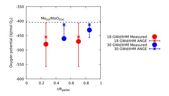
Figure 3.34: Oxygen potential calculated with ANGE compared to values measured by Une et al. [65] at different radial positions at 750 °C. Standard  $UO_2$  fuel. The horizontal dashed line corresponds to the Mo/MoO<sub>2</sub> redox system.
