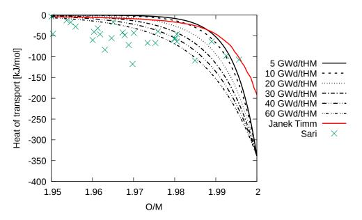
Figure 4.33: Heat of transport in  $UO_2$  fuels irradiated up to different burnups as a function of the O/M ratio compared to the model proposed by Janek [108], based on a reassessment of Sari's measures [106].
