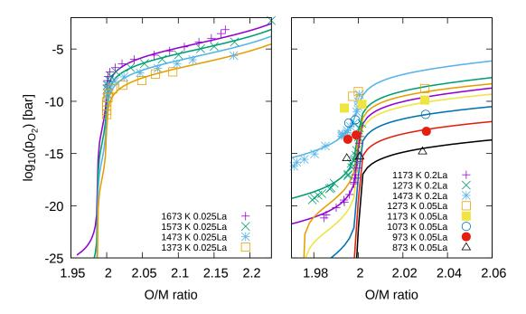
Figure 3.23: Calculated oxygen partial pressure in  $U_{1-y}La_yO_{2\pm x}$  (lines) as a function of O/M, temperature and La mole fraction compared to measured values (symbols). Experimental data from [174–176].
