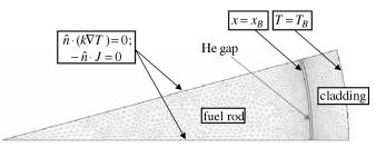
Figure 4.12: FE mesh of the fuel rod fragment simulated by Ramirez et al. Adapted from Ramirez et al. [81].
