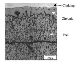
Figure 2.10: Zirconia layer on the cladding inner wall observed in a  $UO_2$  fuel rod after 5 cycles [60].
