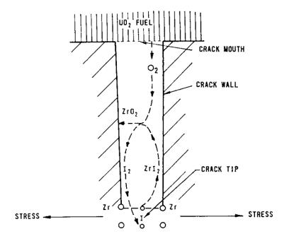
Figure 2.31: Mechanism of SCC assuming presence of gaseous iodine [23].
