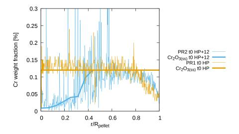
Figure 5.20: Calculated Cr weight fraction evolution during the holding period compared to EPMA measurements after PR1 and PR2.
