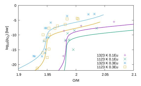
Figure 3.25: Calculated oxygen partial pressure in  $U_{1-y}Eu_yO_{2\pm x}$  (lines) as a function of O/M, temperature and Eu mole fraction compared to measured values (symbols). Experimental data from [43].
