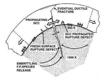
Figure 1.15: Schematic representation of of PCI in 2D. Adapted from [25].
