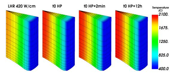
Figure 5.15: Calculated temperatures [°C] in the fuel fragment at different times during the power ramp PR2.
