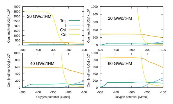
Figure 3.33: Concentrations of volatile species important in SCC as a function of oxygen potential at 2000  $^{\circ}$ C. Fuels irradiated to 20, 40 and 60 GWd/tHM. Elemental compositions used in the calculations are given in Table 3.17.
