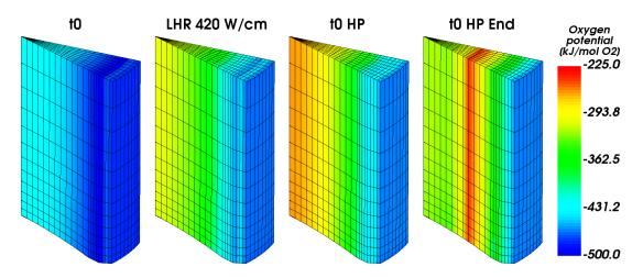
Figure 5.35: Oxygen potential calculated at different moments of PR5.
