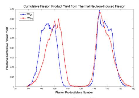
Figure 1.6: Fission product yields of  $^{235}$ U and  $^{239}$ Pu for thermal neutrons. Horizontal axis expresses the mass number and the vertical one presents the fractional cumulative fission yield. Adapted from Dayman et al. [9]
