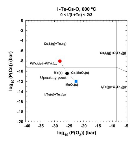
Figure 2.13: Cs-I-O-Te gas phase diagram at 600 °C with the assumption that  $0 < \frac{I}{I+Te} < \frac{2}{3}$ . The red and blue points refer to the experiments studied by Desgranges et al. Figure adapted from [61].
