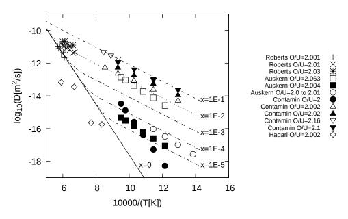
Figure 4.37: Self-diffusion coefficient based on the work of Berthinier [91] compared to experimental data [92, 93, 96, 192, 193]. Hyperstoichiometric domain.
