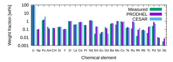
Figure 3.11: PRODHEL calculations of the integral weight fractions of chemical elements compared to ICP-MS measurements from Walker et al. [7] and to CESAR calculations.
