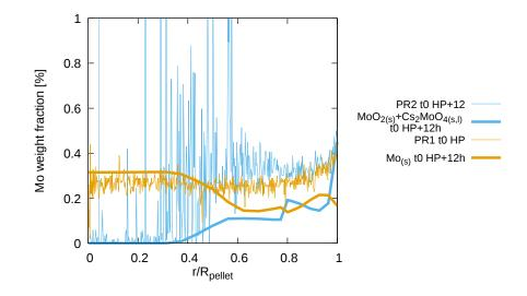
Figure 5.23: Calculated molybdenum oxides  $MoO_{x(s,l)}$  and metallic molybdenum  $Mo_{(s)}$  weight fraction evolution during the HP of power ramp PR1 compared to EPMA measurements after power ramps PR1 and PR2. PR1 rodlet has a lower burnup than PR2 rodlet so the Mo weight fraction is lower on average.
