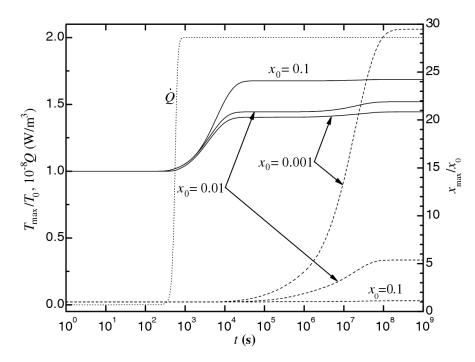
Figure 4.13: Results of the COMSOL Multiphysics simulation. Solid lines:  $T_{max}/T_0$ , dashed lines:  $x_{max}/x_0$ , dotted line:  $\dot{Q}$ . Adapted from Ramirez [81].
