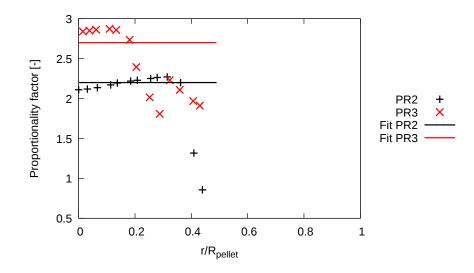
Figure 5.7: The proportionality factor  $\alpha$  of PR2 and PR3 at the pellet center. The lines are the average values for  $r/R_{pellet} < 0.2$ .
