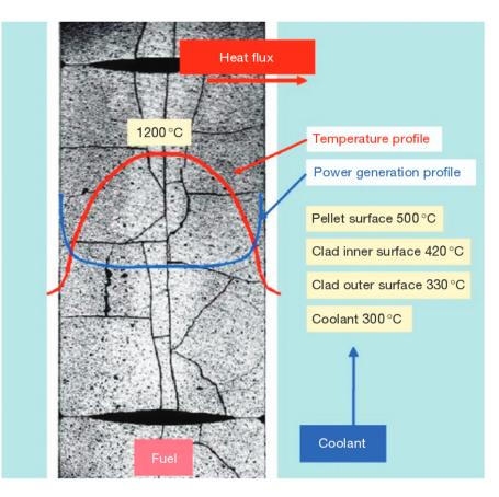
Figure 1.3: "Temperature profile in light water reactor fuel during base irradiation." Adapted from Baron and Hallstadius [3].
