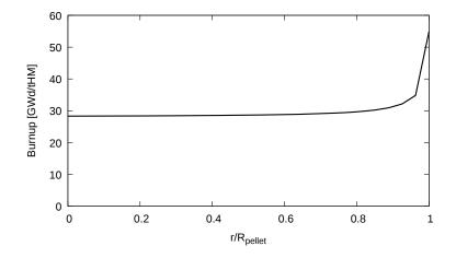
Figure 3.7: Calculated burnup radial profile of PR1.
