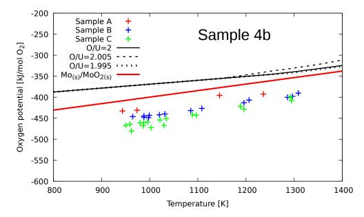
Figure 3.40: Calculated oxygen potential compared to experimental measurements from Matzke [66]. Burnup 200 GWd/tHM. O/U refers to the initial composition.
