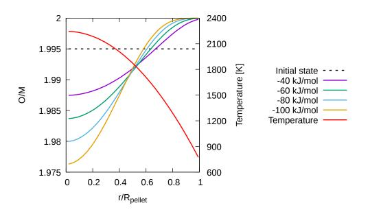
Figure 4.3: O/M profiles calculated by OXIRED for different heats of transport. The red curve is the temperature radial profile.
