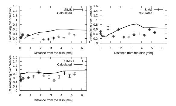
Figure 5.41: Comparison of the calculated axial profiles of Cs, I and Te to the SIMS measurements at r/R=0.1 at the end of PR5. The experimental error is estimated to be 10%.
