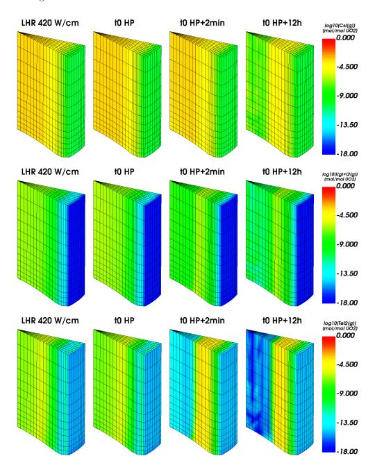
in the fuel pellet fragment leads to the formation of  $CsI_{(g)}$ , as can be seen from the 3D plots of Figure 5.27.
