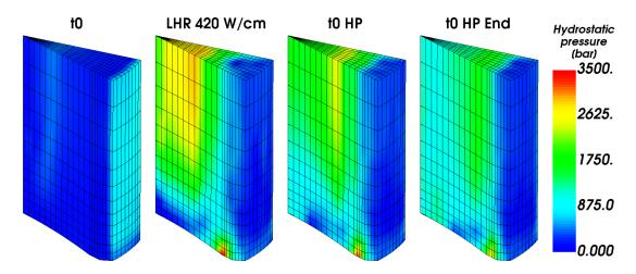
Figure 5.33: Hydrostatic pressure [bar] calculated at different times during PR5.
