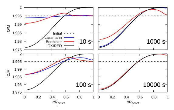
Figure 4.44: Oxygen redistribution calculated with different chemical oxygen diffusion coefficients compared to the steady state redistribution calculated with OXIRED.
