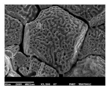
Figure 1.12: Micrograph showing tunnels on the grain face of fuel irradiated up to 22 GWd/tHM [18]. Sample power ramped in the Halden Reactor. Maximum temperature 1800  $^{\circ}$ C, holding time 1800 s.
