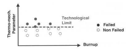
Figure 1.16: PCI technological limit [28].
