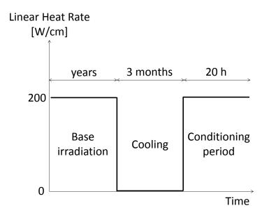
Figure 3.3: Schematic representation of the power sequence used in the iodine isotopic evolution during the conditioning period.
