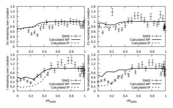
Figure 5.40: Comparison of the calculated radial profiles of Xe, Cs, I and Te to the SIMS measurements along the mid-pellet plane at the end of PR5. The experimental error is estimated to be 10%. MP-Mid Pellet, IP-Inter Pellet.
