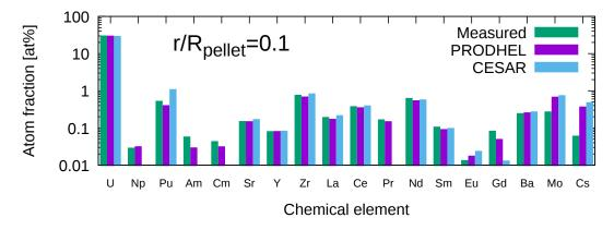
Figure 3.13: PRODHEL calculations of the local atom fractions of chemical elements compared to EPMA measurements from Walker et al. [7] and to CESAR calculations at  $r/R_{pellet}=0.1$ .
