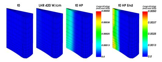
Figure 5.45: Concentration [mol/mol UO<sub>2</sub>] of  $Cs_{(g)}+2Cs_{2(g)}$  at different times during PR5. Note the different scales.
