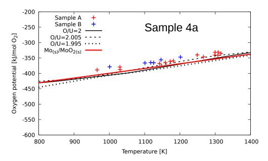
Figure 3.39: Calculated oxygen potential compared to experimental measurements from Matzke [66]. Burnup 75 GWd/tHM. O/U refers to the initial composition.
