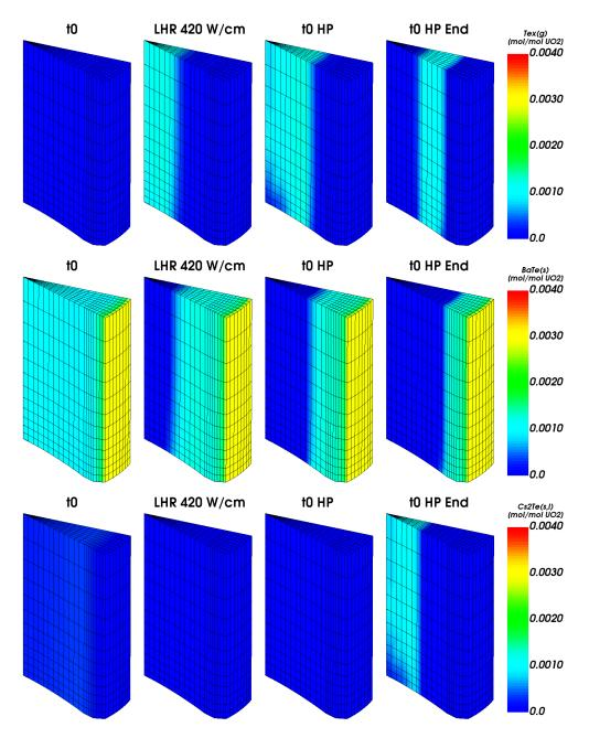
Figure 5.47: Concentrations [mol/mol UO<sub>2</sub>]  $\operatorname{Te}_{x(g)}$  (top),  $\operatorname{BaTe}_{(s)}$  (middle) and  $\operatorname{Cs}_2\operatorname{Te}_{(s,l)}$  (bottom) at different mtimes during PR5. Te<sub>x</sub> stands for different forms of gaseous Te  $(1 \leq x \leq 5)$
