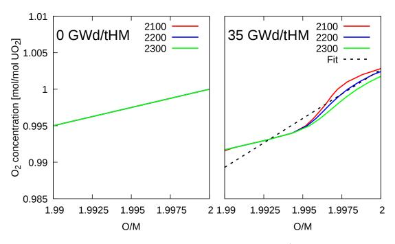
Figure 5.3: Oxygen concentration as a function of the O/M ratio at different temperatures. Left figure–fresh fuel, right figure–fuel irradiated to 35 GWd/tHM. Calculations done with ANGE.
