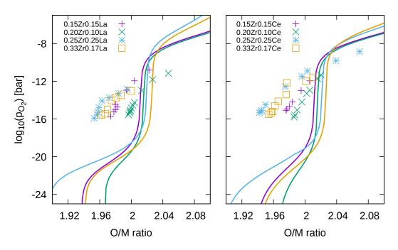
Figure 3.26: Calculated oxygen partial pressure in  $U_{1-y-z}Zr_yLn_zO_{2\pm x}$  (lines) as a function of O/M and mole fractions of Zr and Ln (Ln=La, Ce) compared to measured values (symbols). Both experiments and calculations performed at 1250 K. Experimental data from [47].
