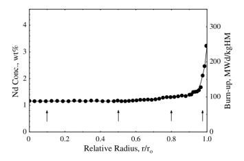
Figure 1.5: Weight fraction of neodymium (left axis) and burnup (right axis) as a function of the relative radius. Measurements come from a  $UO_2$  sample with a very high average burnup of 102 GWd/tHM. Adapted from Walker et al. [7].
