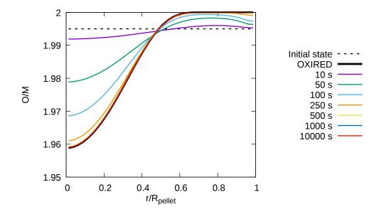
Figure 4.7: O/M radial profiles calculated with OXIRED (thick black curve) and OXITRAN at different times with a nonlinear heat of transport.
