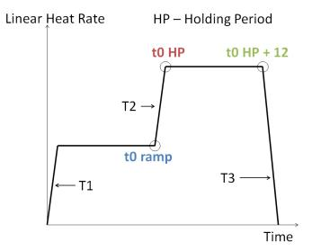
Figure 5.11: Schematic representation of the power ramp test performed by Adamson et al. [73]. The part until "t0 ramp" is the conditioning period. The holding period starts at "t0 HP" and lasts to "t0 HP+12h". Power transients are marked as T1, T2 and T3.
