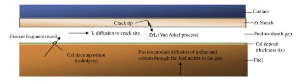
Figure 2.38: Schematic representation of the I-SCC process. Adapted from [115].
