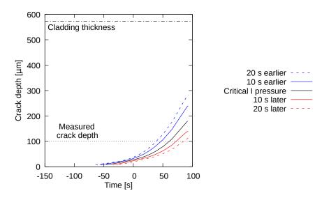
Figure 5.56: Cladding crack depth calculated at the triple point during PR5. Different curves correspond to different activation times for the I-SCC model.
