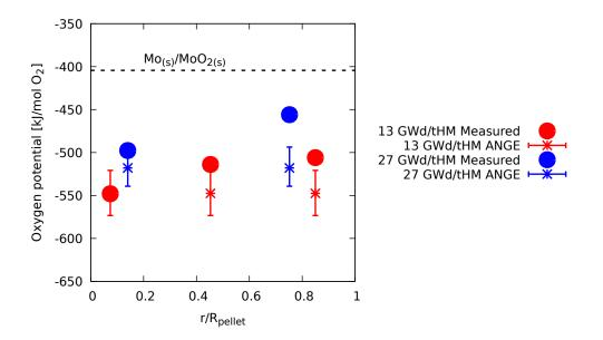
Figure 3.35: Oxygen potential calculated with ANGE compared to values measured by Une et al. [65] at different radial positions at 750 °C.  $2wt\%Gd_2O_3$ -doped fuel. The horizontal dashed line corresponds to the Mo/MoO<sub>2</sub> redox system.
