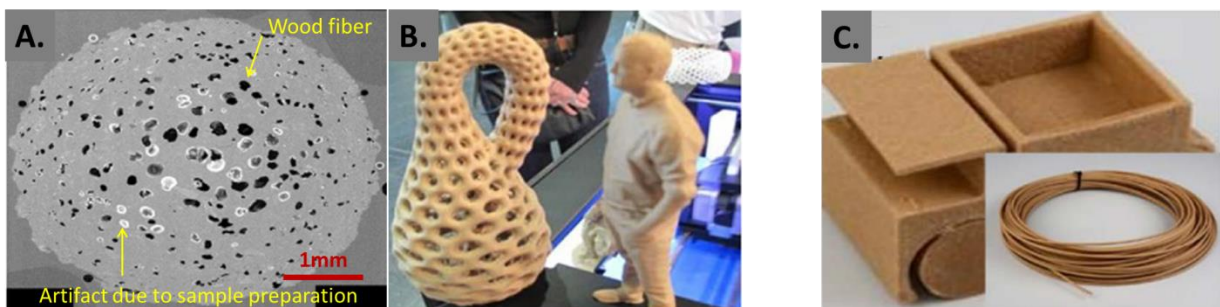
Figure 1-23. 15 wt.% of wood filled PLA: (A) SEM micrograph of a section of the raw filament (Duigou et al. 2016), (B) printed part with WoodFill filament from ColorFabb – 40% of wood filled PLA: (C) Printed part with Laywoo-3D filament from CC-Products (Li T et al. 2016).
