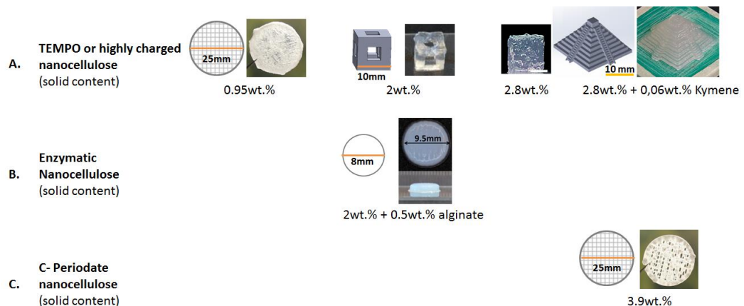
Figure 1-34. 3D printed part with nanocellulose at low solid content. (A) TEMPO or highly charged nanocellulose with increasing solid content from left to right (Rees et al. 2015; Håkansson et al. 2016; V. C. F. Li et al. 2018) (B) enzymatic nanocellulose (Markstedt et al. 2015) and (C) C_Periodate nanocellulose (Rees et al. 2015).
