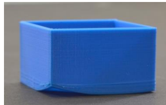
Figure 1-10. 3D printed part with warpage in ABS. According to Simplify 3D troubleshooting guide, ABS material can shrink up to 1.5%.
