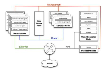
Figure 2.5: Openstack networking overview<sup>3</sup>
