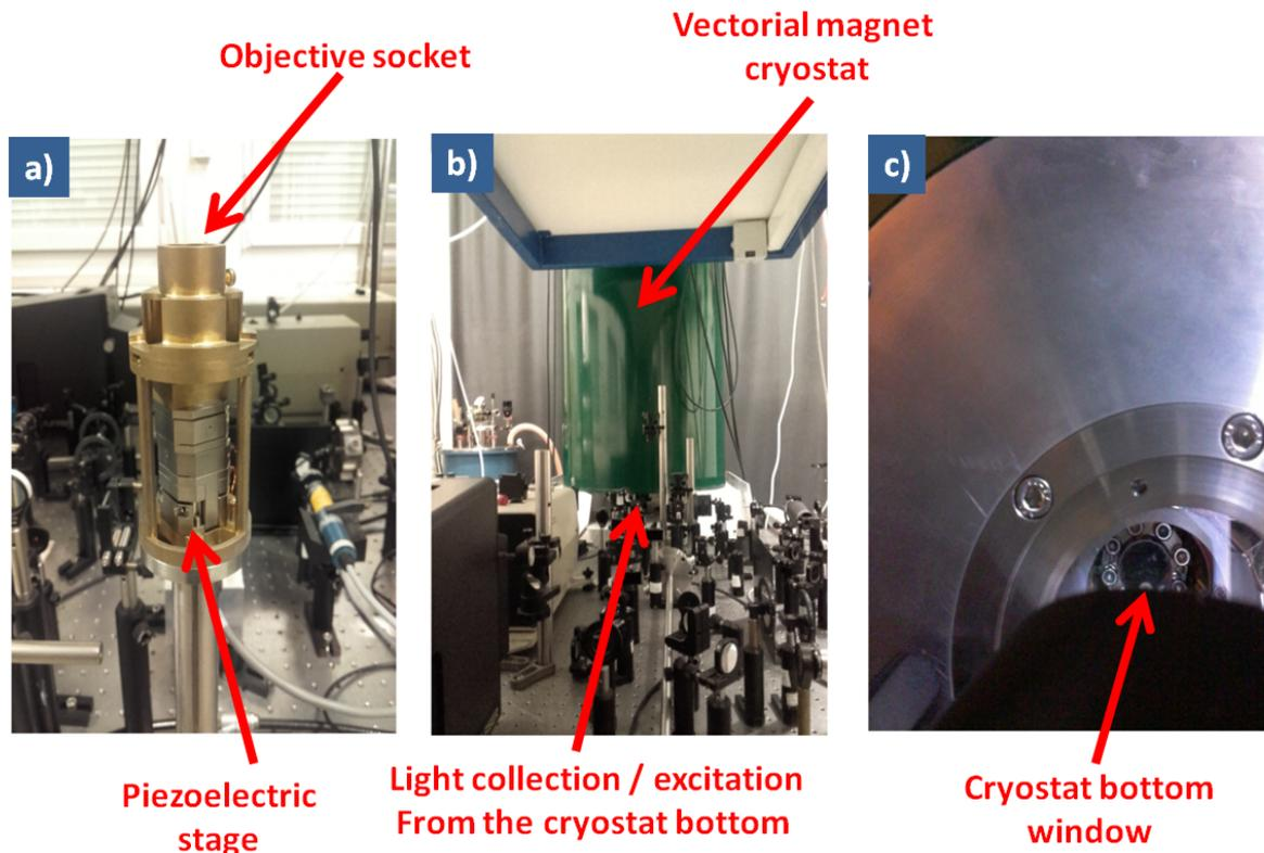
Figure 4.35 – The cryostat transfer rod with the objective and piezoelectric stage assembled a). Picture of the vectorial magnet cryostat b). The window located at the bottom of the cryostat c).
