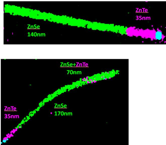
Figure 4.16 – EDX measurements of single nanowires, where along their axis they are composed almost exclusively of ZnSe with some Te inclusions near to the bottom. The nanowire tip is constituted of ZnTe, while at the top we see the catalyst Au droplet.
