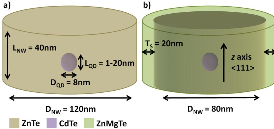
Figure 2.7 – The configuration of the two different nanowire quantum dots studied. A CdTe quantum dot inserted in a ZnTe nanowire a) and a CdTe quantum dot inserted in a ZnTe nanowire passivated by a ZnMgTe shell
