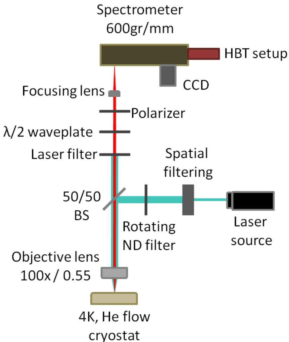
Figure 4.2 – Schematic representation of the micro-photoluminescence setup we used for the basic optical characterization of the nanowire quantum dots.
