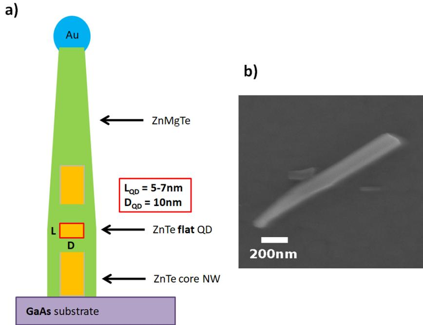
Figure 4.5 – Schematic representation of an as-grown ZnMgTe nanowire with a ZnTe core and a ZnTe flat quantum dot a). An SEM image of the actual nanowire dispersed on a Si substrate in order to carry out the micro-photoluminescence measurements b).
