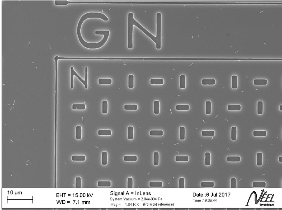
Figure 4.4 – A typical SEM image showing the patterned Si substrate with the dispersed nanowires, which we use in order to navigate and select the nanowires on which we perform the optical measurements.
