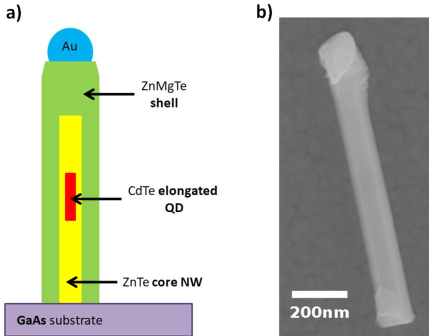
Figure 4.18 – Schematic representation of the cross section of an as-grown ZnTe-ZnMgTe core-shell nanowire, incorporating an elongated CdTe quantum dot a). SEM image of a dispersed nanowire on a Si substrate similar to those we carried out the micro-photoluminescence measurements b).
