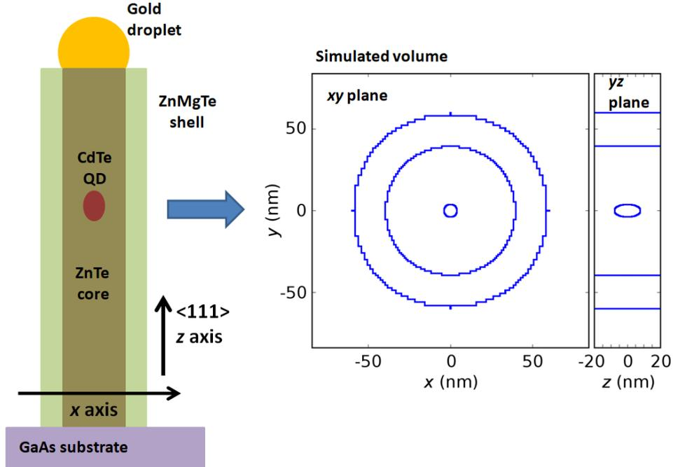
Figure 2.4 – Schematic representation of the actual nanowire quantum dot structure (left) and the section we define for the numerical calculation (right).
