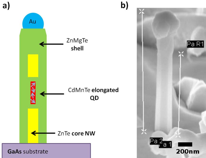
Figure 4.20 – Sketch of the cross section of an as-grown ZnTe-ZnMgTe core-shell nanowire, with an elongated CdMnTe quantum dot, surrounded by ZnMgTe a). SEM image of the as-grown sample showing a nanowire similar to that we performed the micro-photoluminescence measurements.
