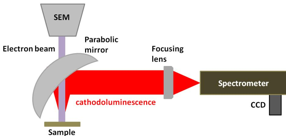
Figure 4.3 – Schematic representation of the cathodoluminescence setup.
