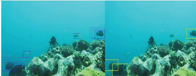
Fig. 5. Results of the detection before (left) and after (right) post-processing. Note that two fishes in the center are not displayed because they do not belong to one of the species which have been learned.
