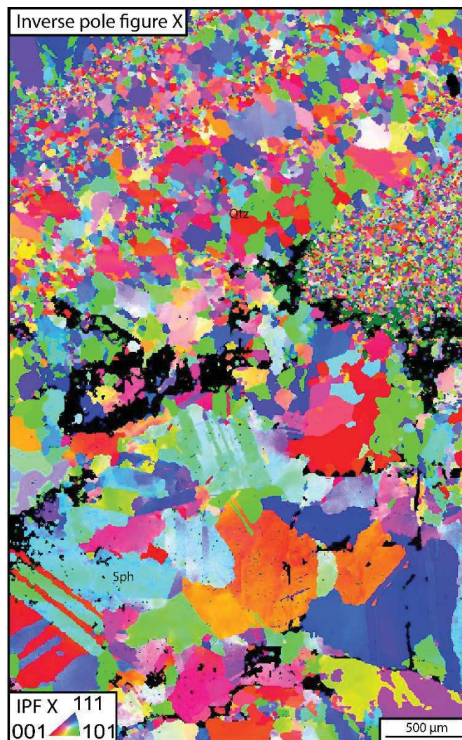
Figure 157. EBSD map of Liat stratabound sphalerite ( 6\ \mu\text{m} = step of measurement, same area as Figure 156) with inverse pole figure according to the X.
