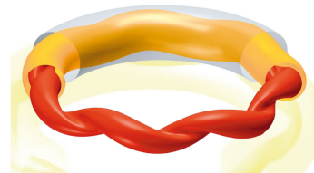
Figure 1.4: Schematic figure of the helical magnetic field in RFP.
