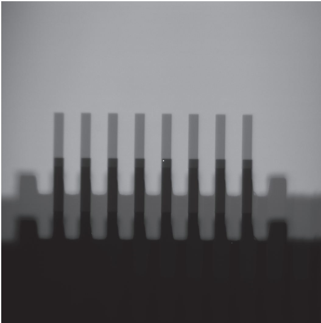
Figure 5.28 Image of a \mu cantilever sample from the CryoQPDI camera. The \mu cantilevers nominal dimensions are 500 \times 90 \times 1 \mu\text{m} . The bright dot on the fifth \mu cantilever (from left to right) is the laser spot of the interferometer. As shown in figure 2.1, page 14, the laser beam of the interferometer is separated in two beams on its forward path to the sample. The image on the camera, observed on the beam return path, displays a reciprocal situation. As the beams are recombined by the Semel-Savart plate, only a single spot is visible. The light coming from the \mu cantilevers, which is not polarized in a particular direction relative to the Semel-Savart plate axes, is however split in two by the beam splitter. In other words, instead of a \mu cantilever with two laser spots, the image acquired by the camera displays a single spot with two \mu cantilevers. Looking at one of the \mu cantilever image at a time, one can indeed infer the position of the reference beam at the base of the \mu cantilever from the top image and the position of the probe beam at the top left corner of the \mu cantilever from the bottom image.
