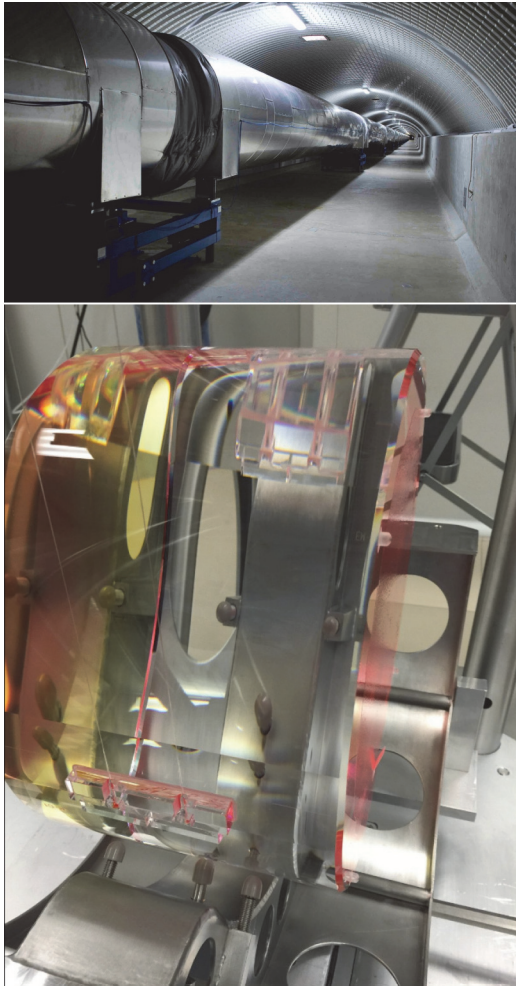
Figure 1.8 Illustration of Advanced VIRGO construction [27]. On the top left: vacuum tube of one of the interferometer arms. Bottom left: suspension of a mirror. Notice the two very thin glass wires suspensions attached to the mirror side. They are employed to reduce the suspension thermal noise. Right: the superattenuator is a multistage mechanical filter intended for an aggressive attenuation of the ground vibration.
