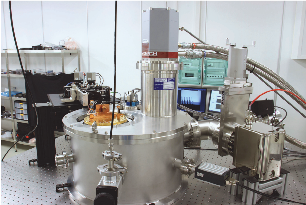
Figure 4.1 Photograph of the CryoQPDI main elements. The cryostat is the main subject of this photograph and is visible at the foreground, while the interferometer sits behind it on the left. From a comparison with the other figures of this chapter, one can recognize from left to right: the main vacuum vessel of the cryostat, the pulse tube connected via two helium gas lines to its compressor (not shown), the pressure sensor and the ion pump. The cold plate is easily identified by its gold color, with the cryo holder attached on it. Apart from the pulse tube compressor and the acquisition and control electronics, all the apparatus sits on an optical table with self-leveling, active air isolator feet.
