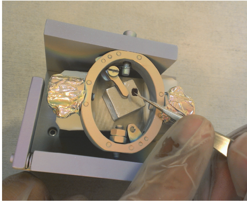
Figure 7.2 Photograph of the first version of the RVDS sample holder. The operator is installing a cantilever sample. Even if a few coating experiments had been conducted successfully using this setup, it quickly showed severe limitations and needed to be replaced by a more reliable design.
