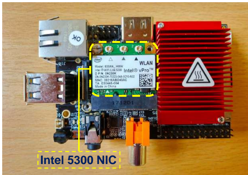
Figure 3.13: The HummingBoard Pro as mobile receiver.
