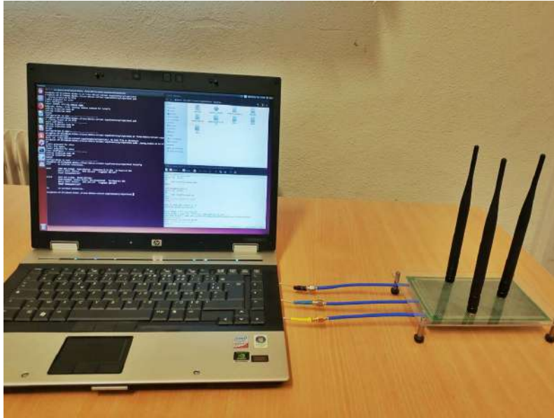
Figure 3.12: The laptop with Intel 5300 NIC as signal transmitter.
