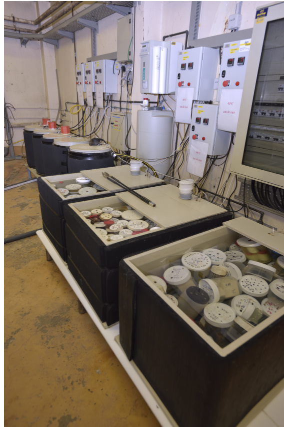
Figure 2.7 – Temperature-controlled seawater ageing baths
