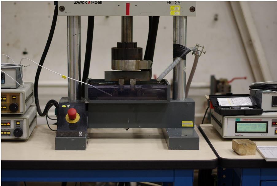
Figure 2.9 – Immersed fatigue four point bending test
