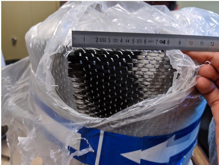
Figure 2.4 – 600 \text{ g/m}^2 carbon fibre fabric with off-axis glass fibre weaving
