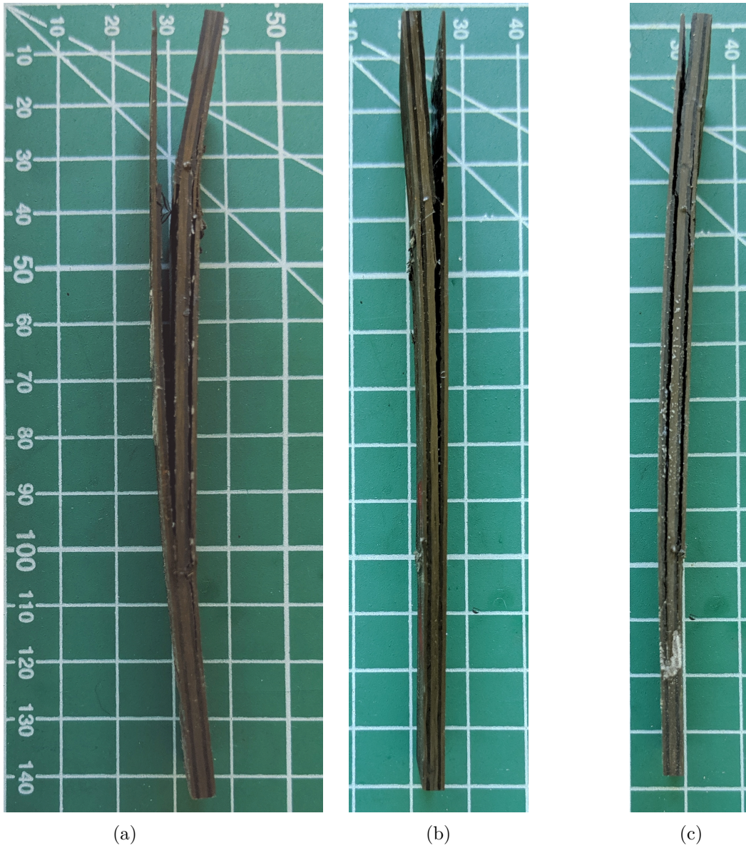
Figure 5.31 – Delamination recorded during fatigue tests for unaged (a), saturated (b) and saturated then dried (c) of infused specimens
