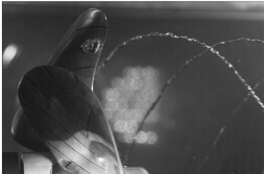
Figure 5 – Example of tip and surface cavitation from [6]
