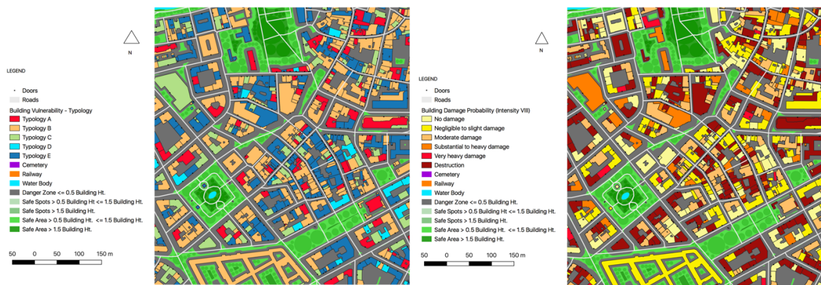
Figure 46 Left: Building Vulnerability – Typology (A to E); Damage: Building Damage (0 to 5) for Intensity VIII Scenario.
