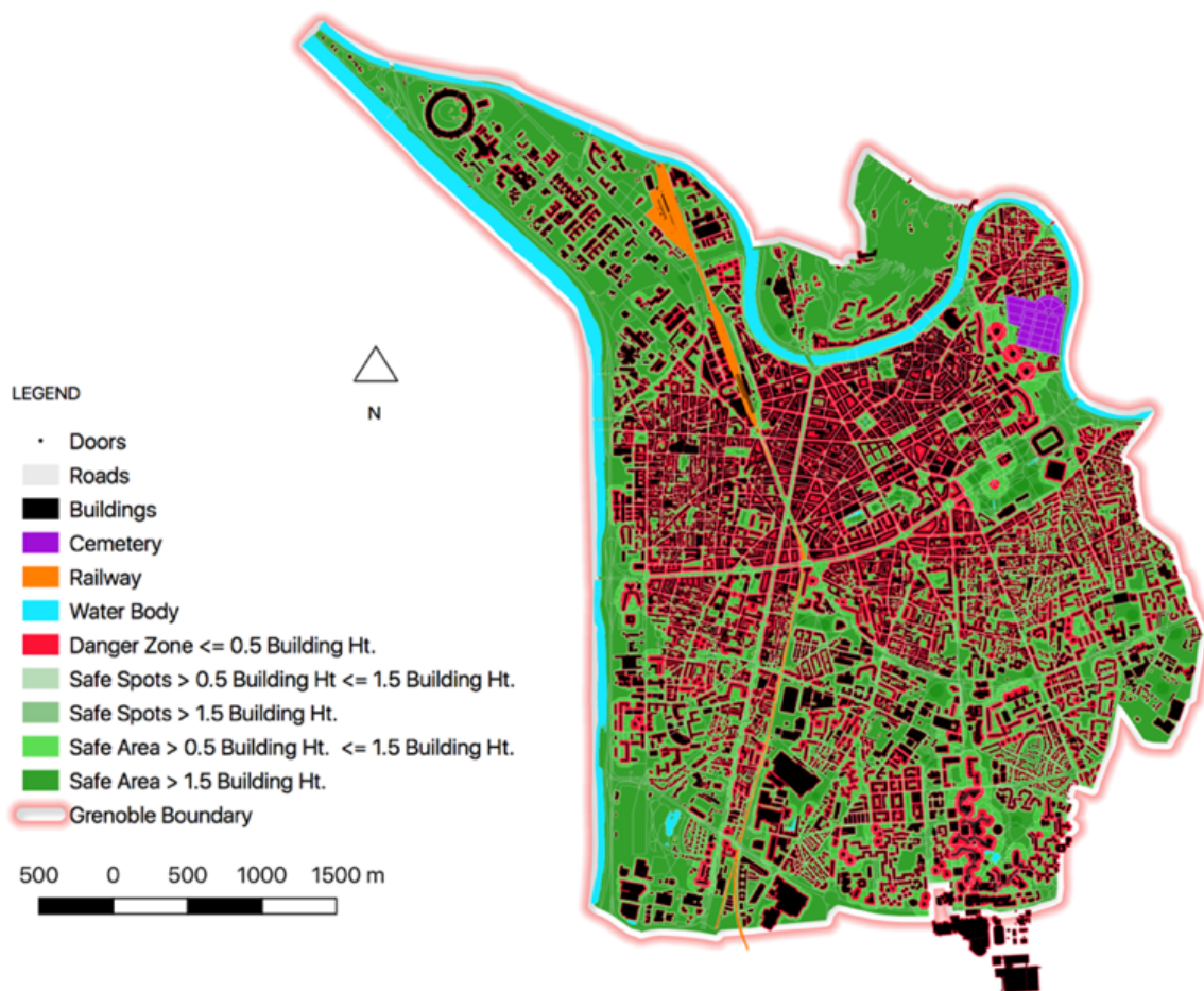
Figure 37 Spatial layers used in the model at the scale of the city of Grenoble
