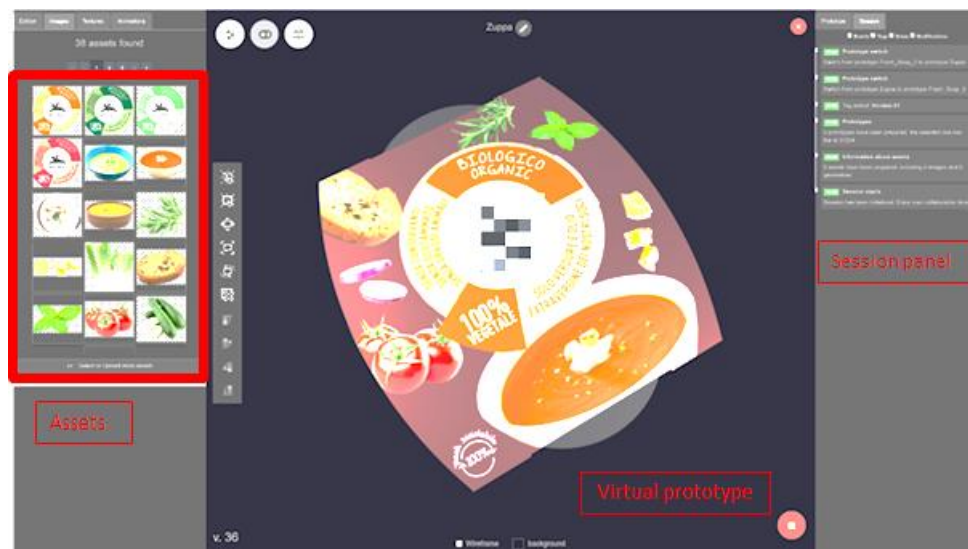
Figure 26. Editing interface of virtual prototype with assets and session panel
