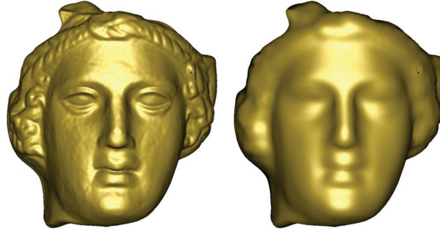
FIGURE 4.1: Both pictures show a rendering of the same shape. The only difference are the normals considered over the shapes. On the left: normals estimated with great precision - On the right: poorly estimated normals
